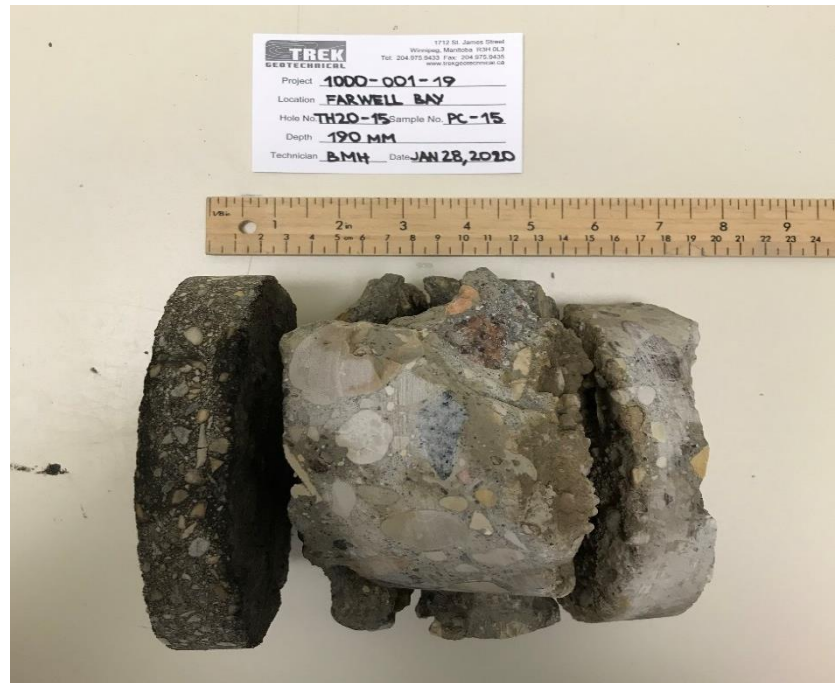
Photo 9: Pavement Core Sample at Test Hole TH20-15
