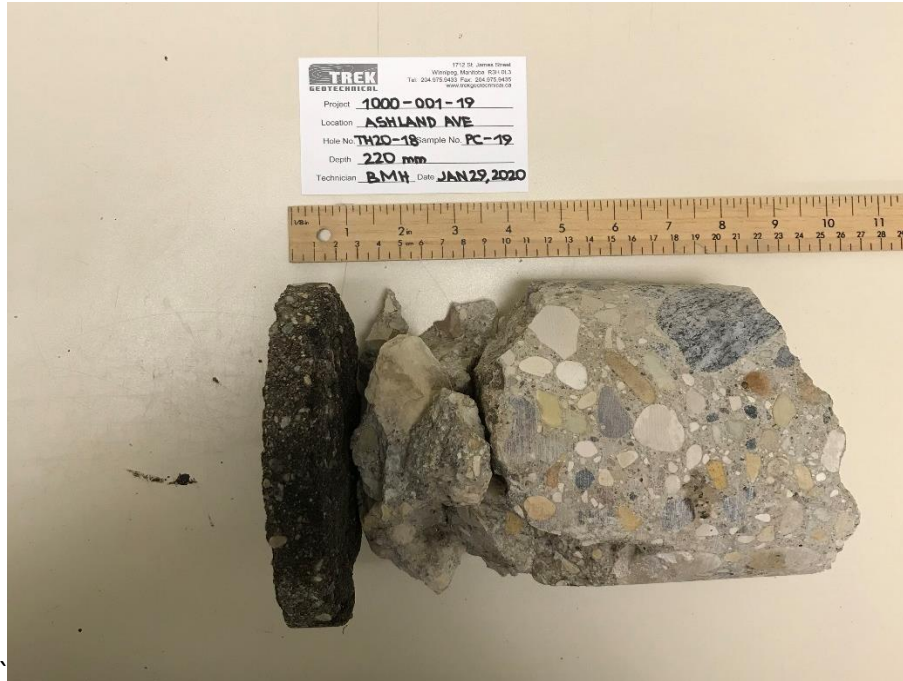
Photo 3: Pavement Core Sample at Test Hole TH20-18
