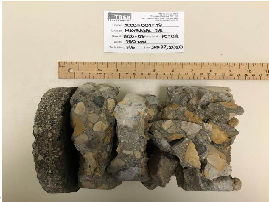
Photo 3: Pavement Core Sample at Test Hole TH20-03
