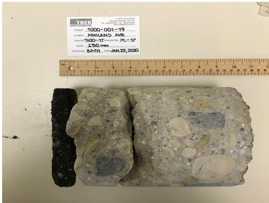
Photo 2: Pavement Core Sample at Test Hole TH20-17
