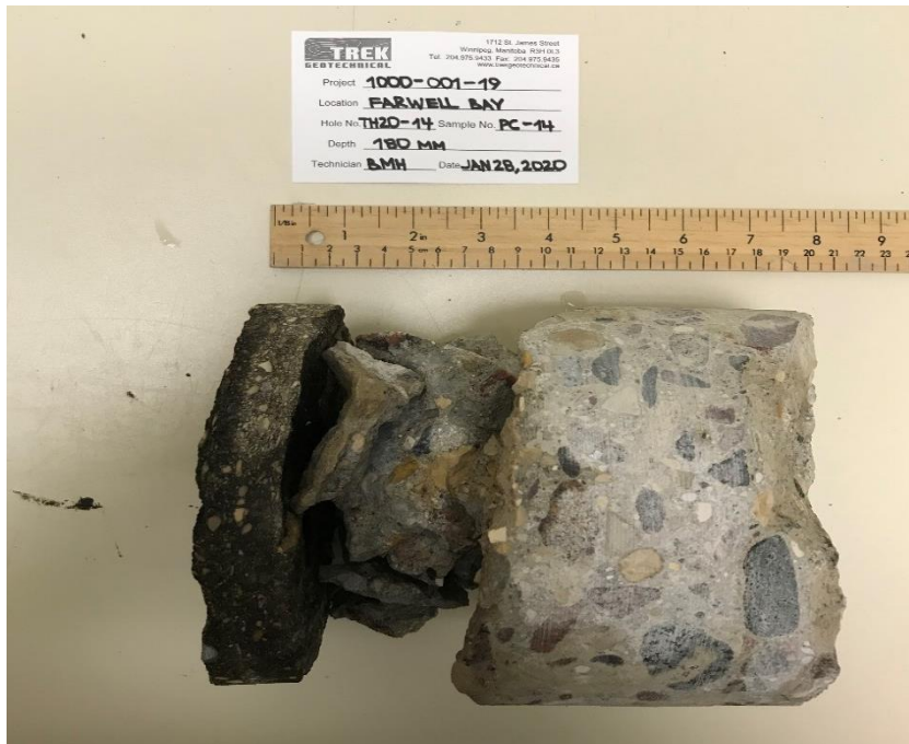
Photo 8: Pavement Core Sample at Test Hole TH20-14
