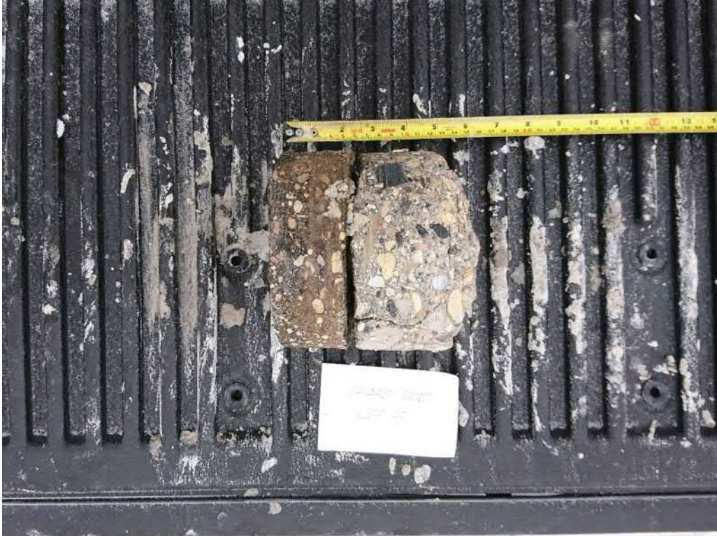
Photograph 7: Core Hole CH20-07 – Sharp Boulevard – Concrete partially recovered
