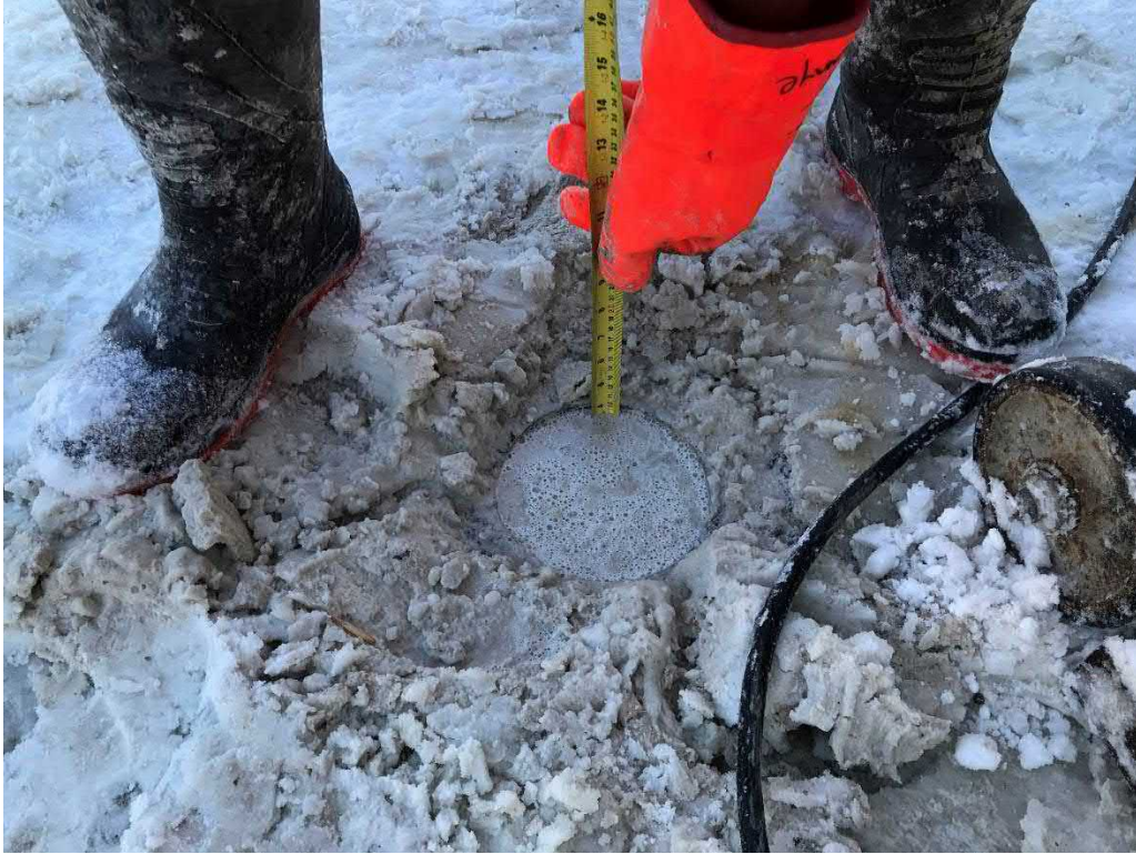
Photograph 15: Core Hole CH20-16 – Colchester Bay – Concrete not recovered, no measurements
