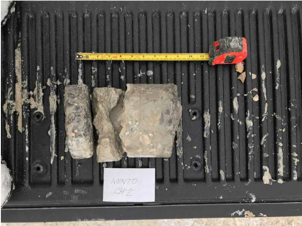
Photograph 2: Core Hole CH20-02 – Minto Street
