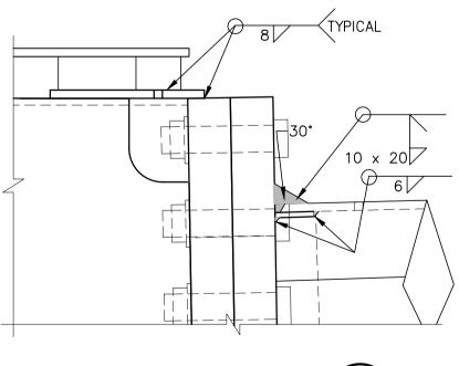
ARM WELD DETAIL SCALE 1:5 3
