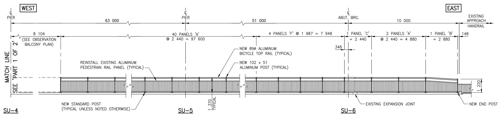
PEDESTRIAN HANDRAIL LAYOUT - PART 2 OF 2 (ELEVATION LOOKING NORTH) SCALE 1:100
