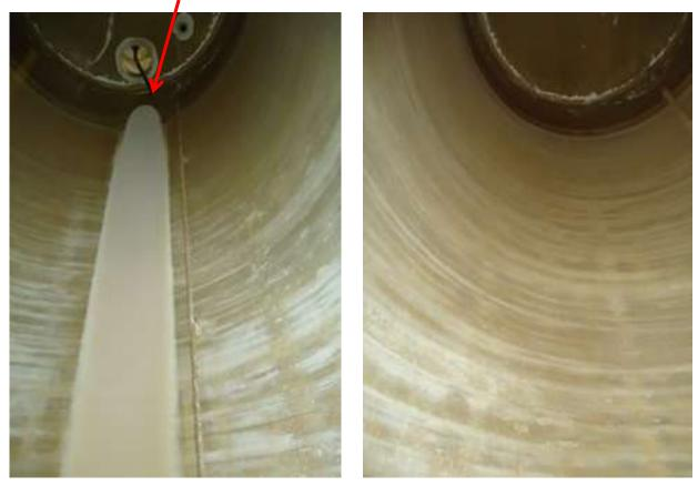
Rotate Inlet towards the center of the tank
