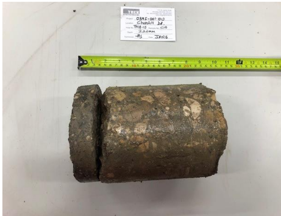
Photo 4: Pavement Core Sample at Test Hole TH17-10
