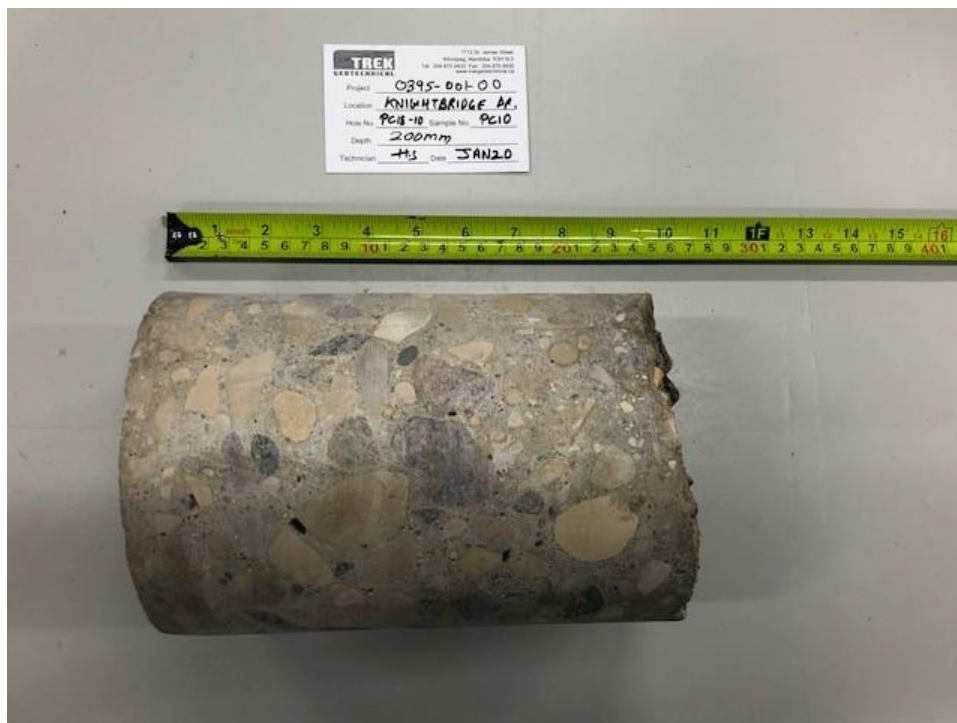
Photo 4: Pavement Core Sample at Test Hole PC18-10
