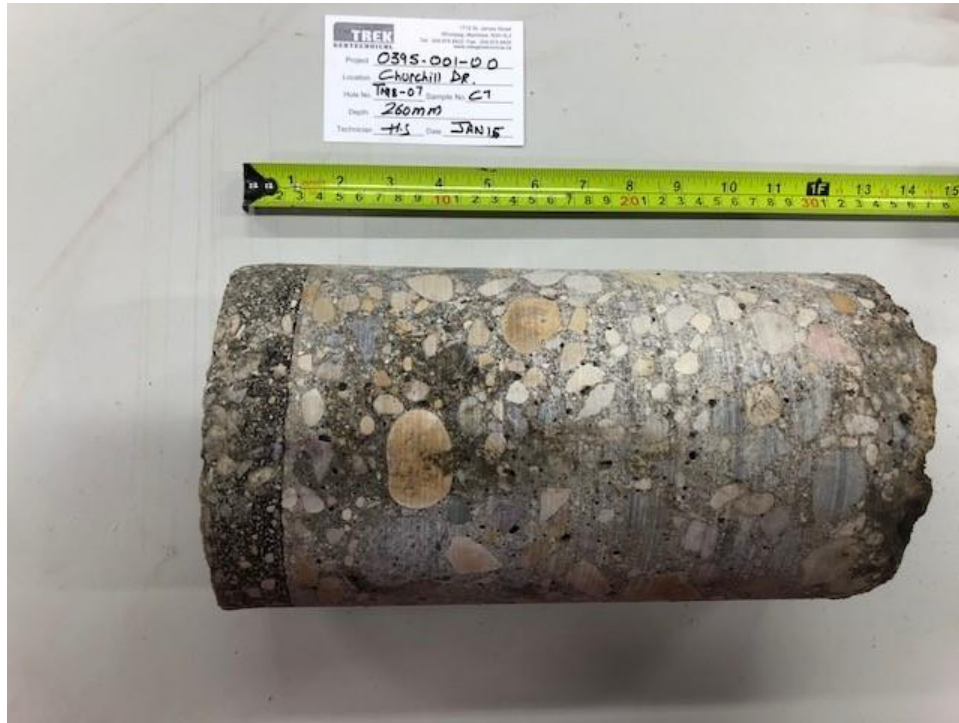
Photo 1: Pavement Core Sample at Test Hole TH17-07
