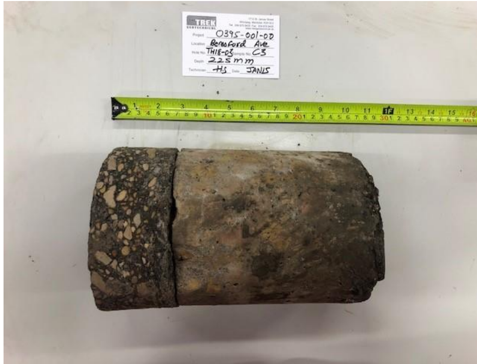
Photo 3: Pavement Core Sample at Test Hole TH17-03
