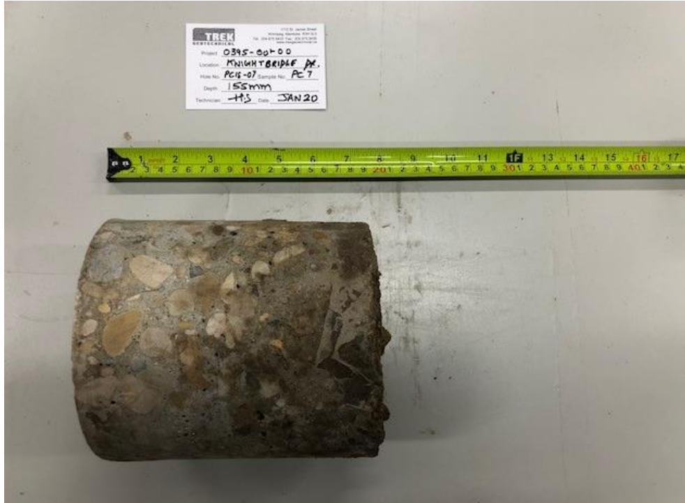
Photo 1: Pavement Core Sample at Test Hole PC18-07
