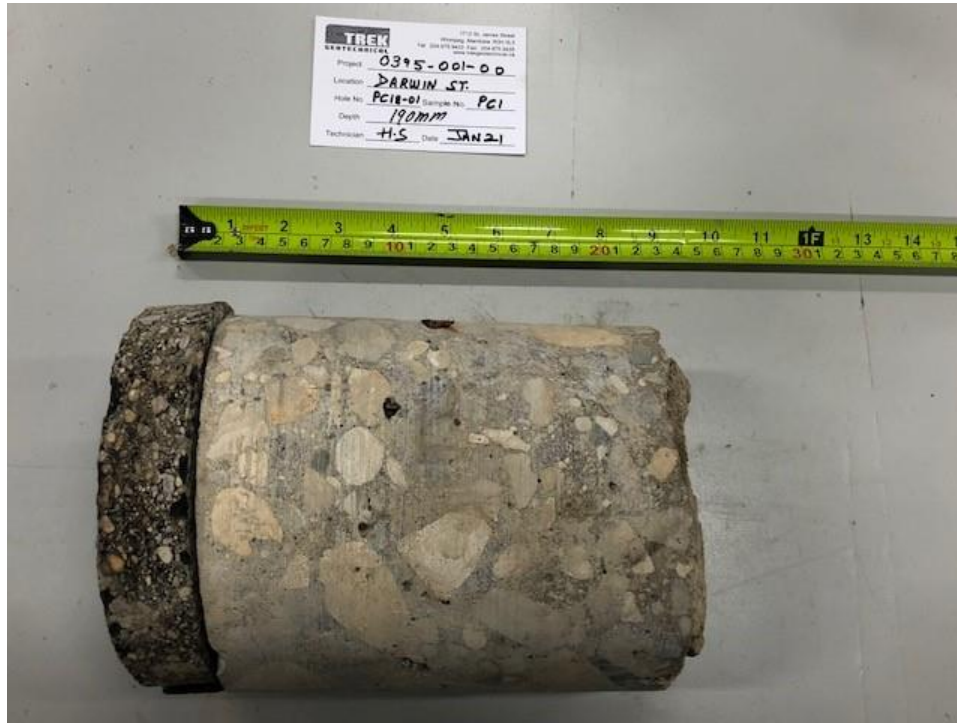
Photo 1: Pavement Core Sample at Test Hole PC18-01
