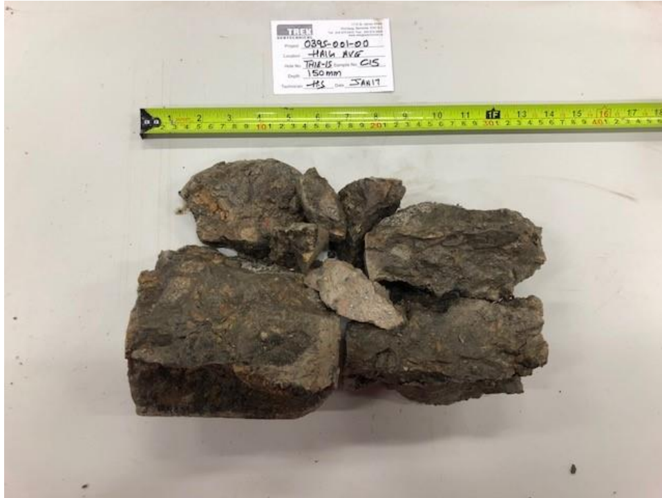
Photo 3: Pavement Core Sample at Test Hole TH17-15
