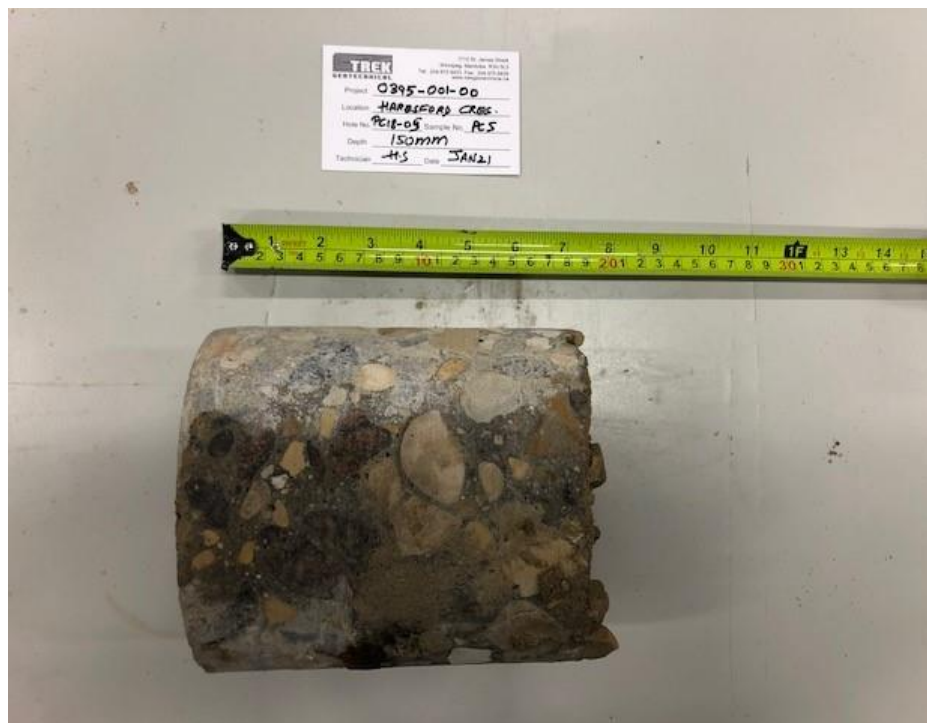
Photo 2: Pavement Core Sample at Test Hole PC18-05
