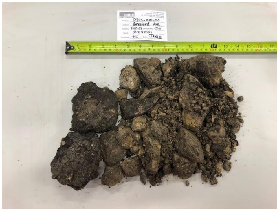
Photo 4: Pavement Core Sample at Test Hole TH17-04
