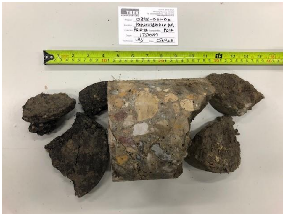
Photo 6: Pavement Core Sample at Test Hole PC18-12
