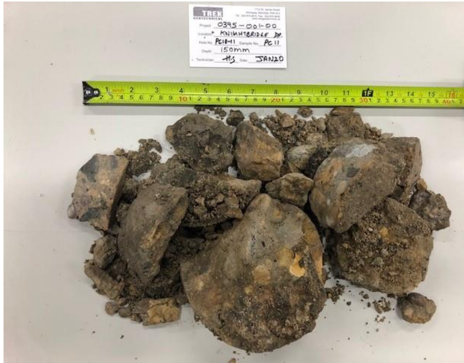
Photo 5: Pavement Core Sample at Test Hole PC18-11
