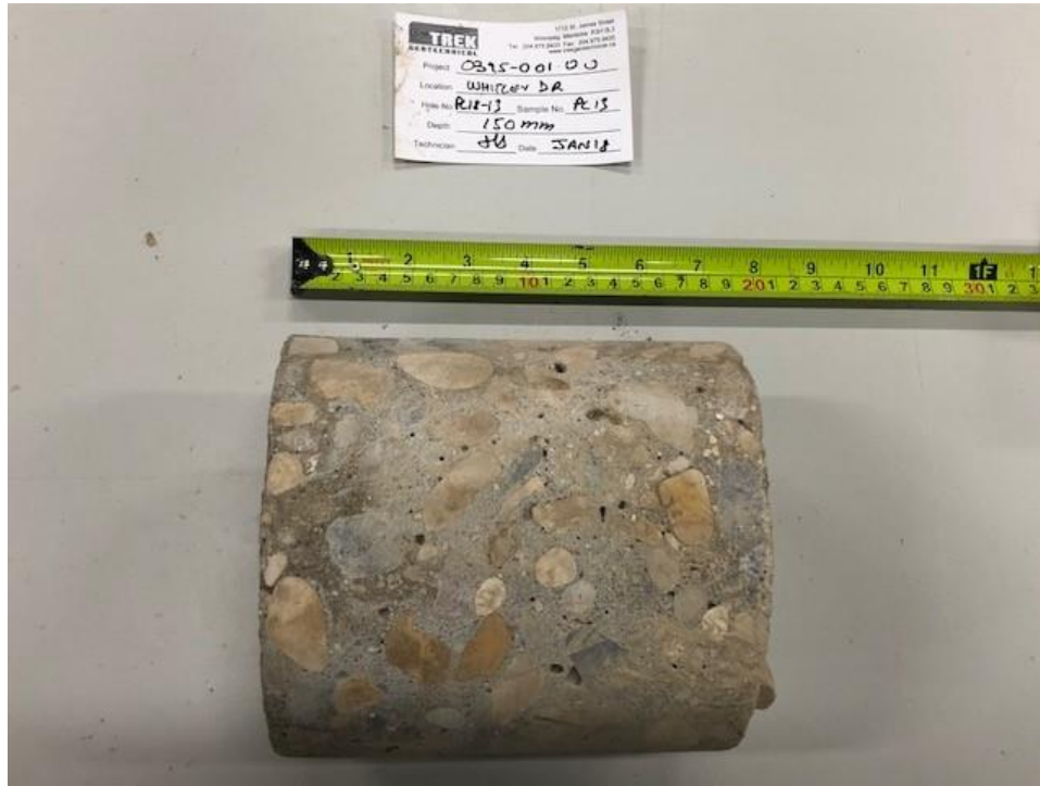
Photo 1: Pavement Core Sample at Test Hole PC18-13
