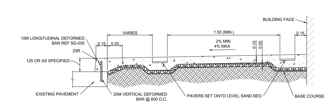
TYPICAL MONOLITHIC CURB AND SIDEWALK - SECTION VIEW N.T.S.
