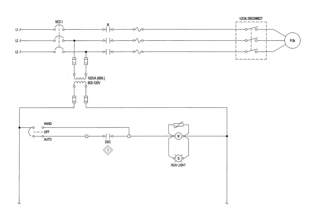
A LAP POOL CIRC. PUMP (P-3A,B) WIRING SCHEMATIC SCALE: N.T.S.
