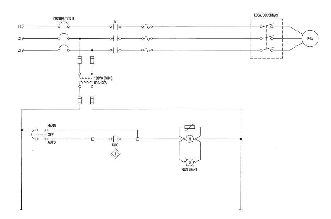
GLYCOL CIRC. PUMP (P-1A,B) WIRING SCHEMATIC SCALE: N.T.S.
