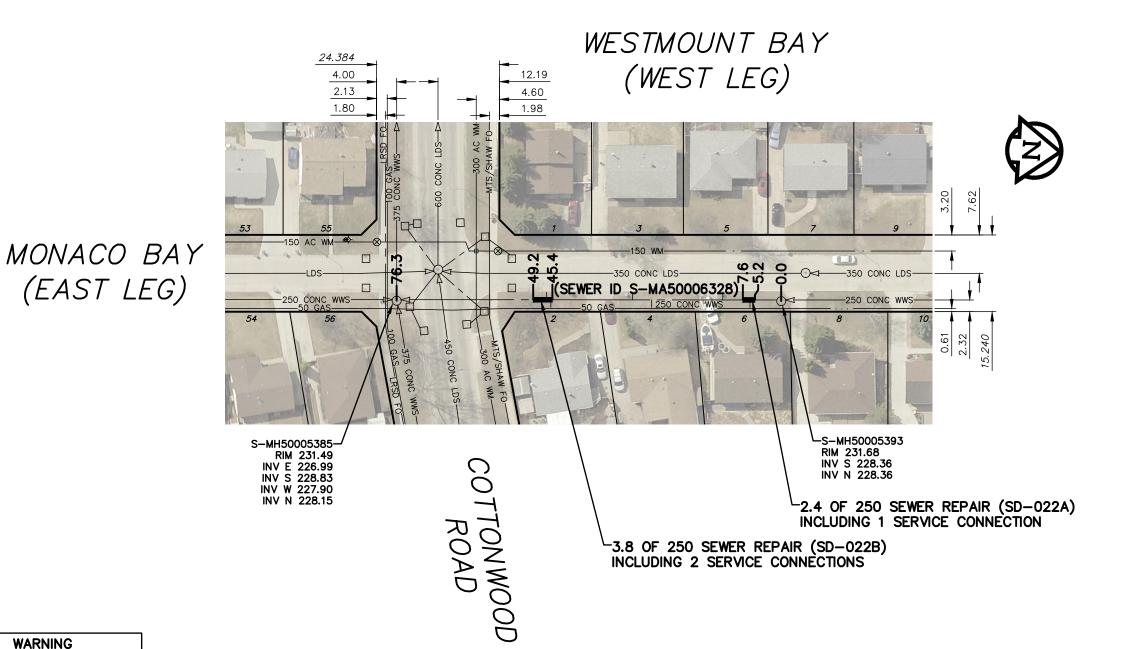
SEWER JUNCTION INFORMATION FROM SEWER VIDEO INSPECTION SEWER ID S-MA50006328 DISTANCE FROM MH S-MH50005393 DIAMETER CLOCK DISTANCE 10 6.2 150 11.6 150 2 25.7 150 10 150 29.5 2 45.7 10 150 46.6 150 2
