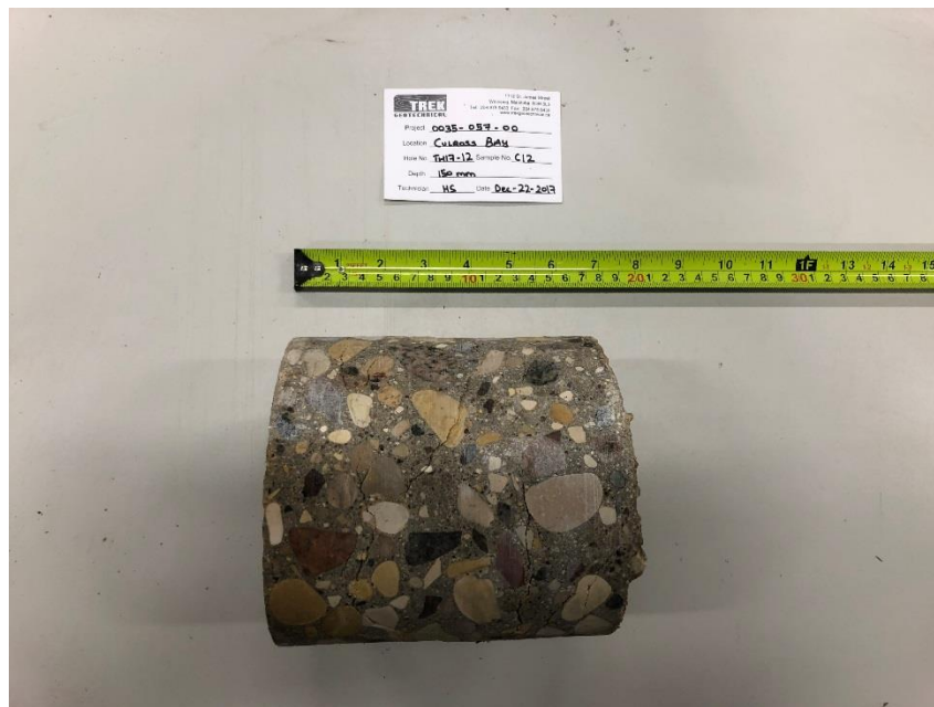
Photo 4: Pavement Core Sample at Test Hole TH17-12
