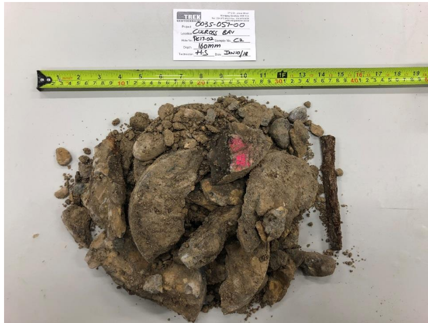
Photo 9: Pavement Core Sample at Pavement Hole PC17-02
