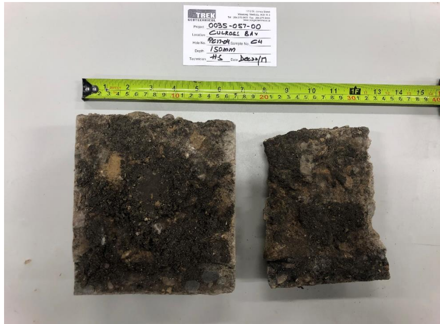
Photo 11: Pavement Core Sample at Pavement Hole PC17-04
