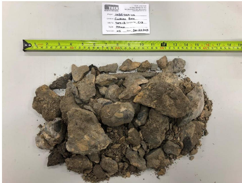
Photo 5: Pavement Core Sample at Test Hole TH17-13
