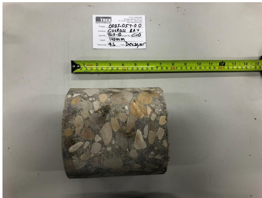
Photo 2: Pavement Core Sample at Test Hole TH17-10
