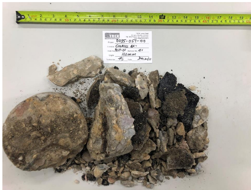
Photo 8: Pavement Core Sample at Pavement Hole PC17-01
