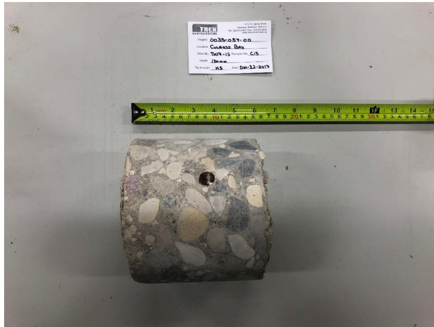
Photo 7: Pavement Core Sample at Test Hole TH17-15
