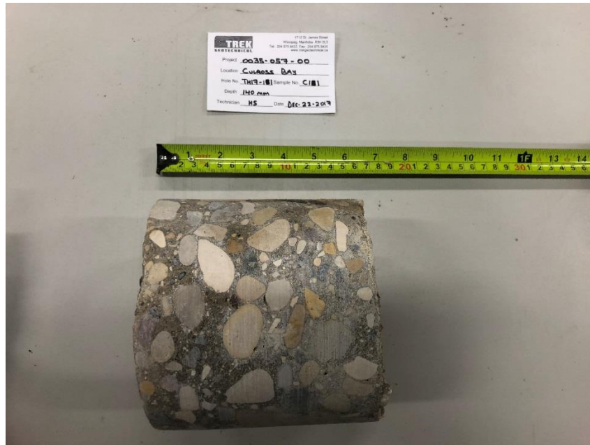
Photo 3: Pavement Core Sample at Test Hole TH17-11
