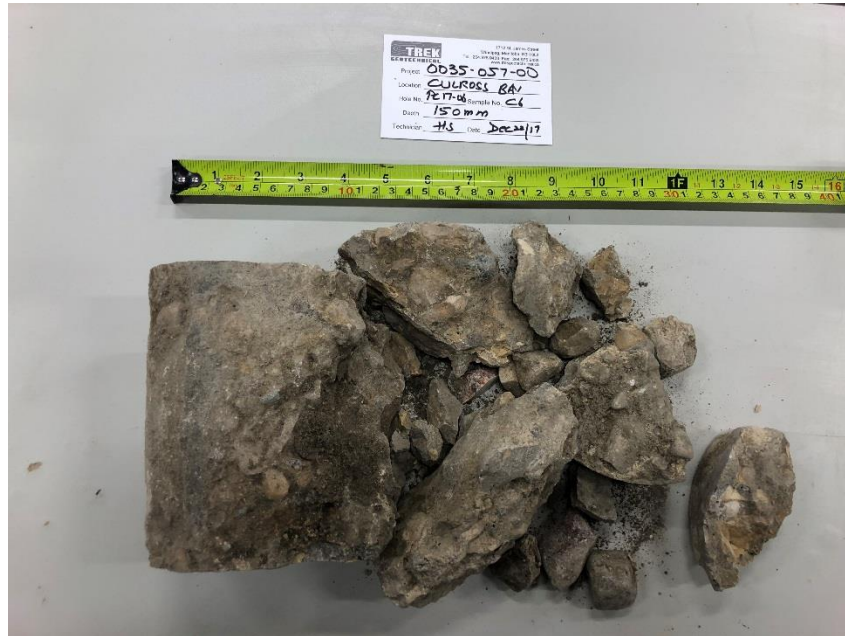
Photo 13: Pavement Core Sample at Pavement Hole PC17-06
