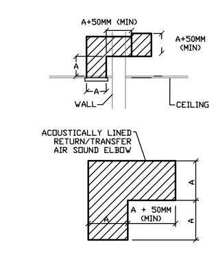
2 ACOUSTIC ELBOW DETAIL M5.1 | SCALE: NTS
