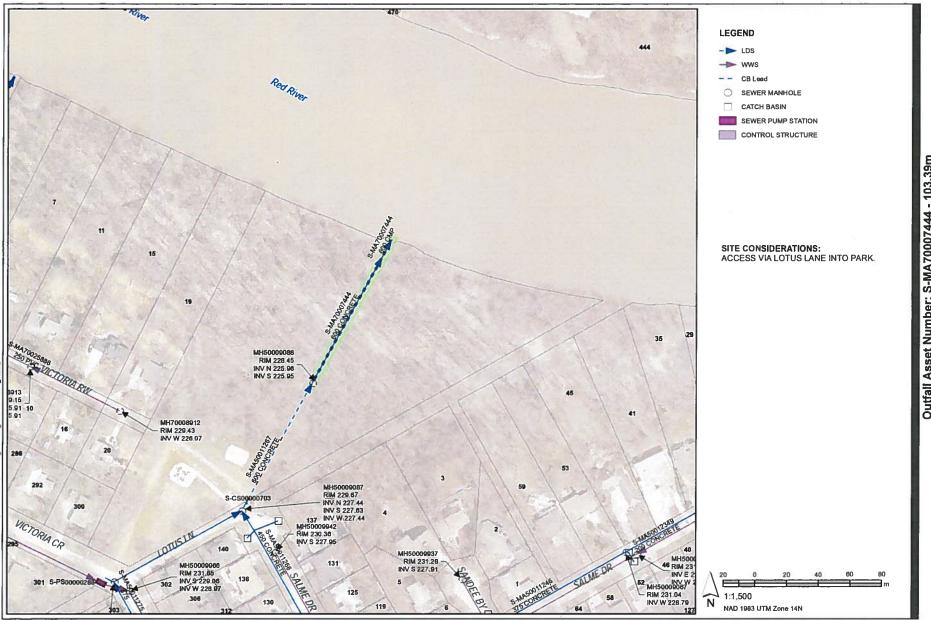
Outfall Asset Number: S-MA70007444 - 103.39m Upstream Sewer Asset Number: None - 0m Upstream Manhole Coordinates: 634666.2884E, 5522585.7339N Location: 19 VICTORIA ROW
