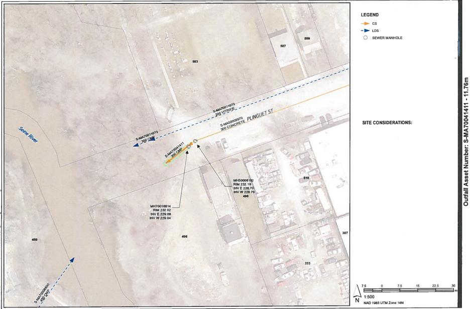
Outfall Asset Number: S-MA70041411 - 11.76m Upstream Sewer Asset Number: None - 0m Upstream Manhole Coordinates: 636095.9541E, 5528394.7429N Location: 503 RUE PLINGUET
