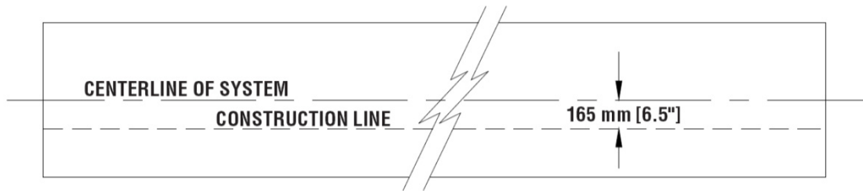
Figure 46 (Top view of concrete foundation)
