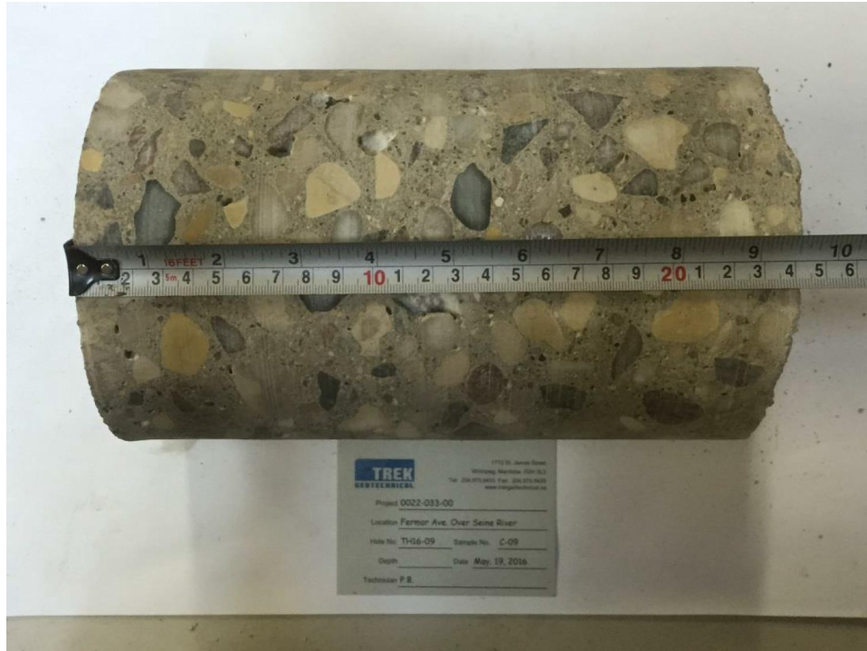
Photo 9: Pavement Core Sample at Test Hole TH16-09
