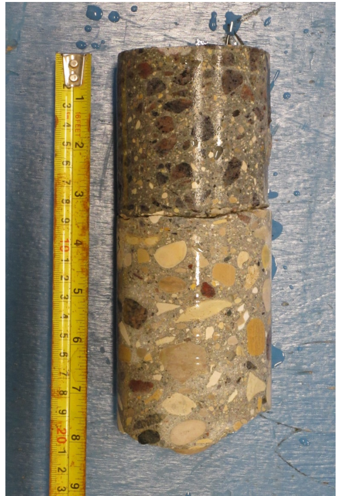
Figure 4 – Core no. D4, eastbound curb lane
