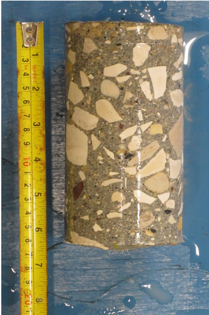
Figure 27 - Core no. A7, west abutment
