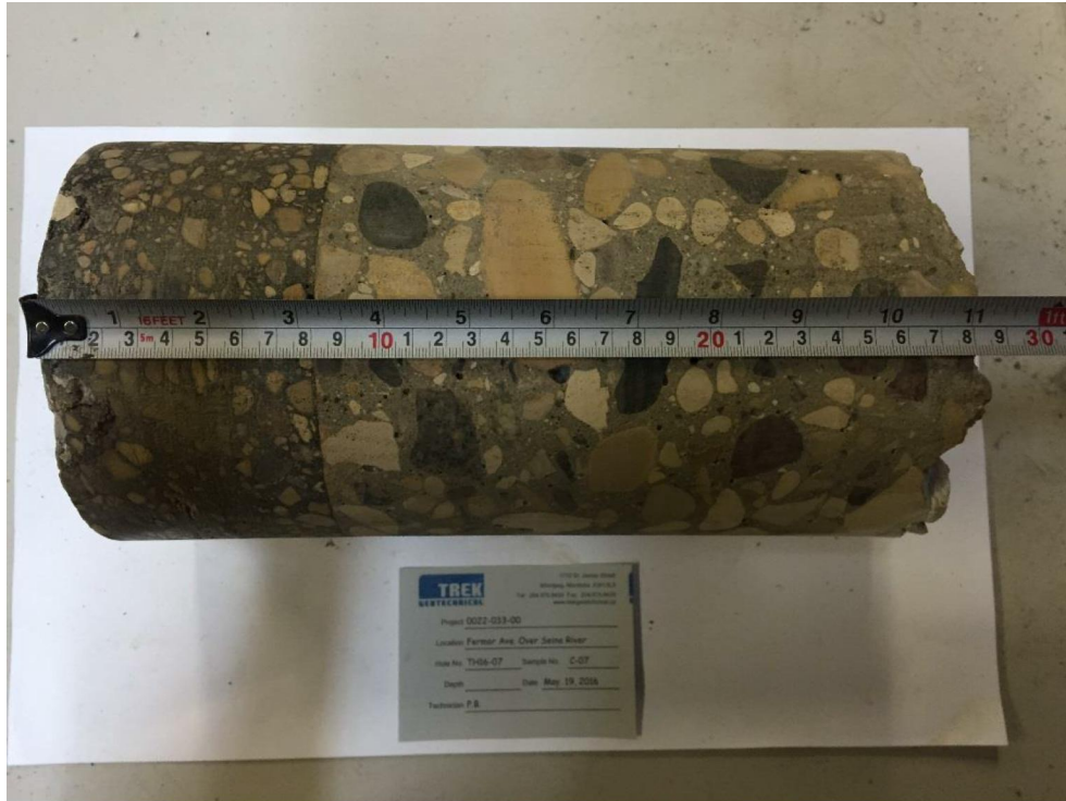
Photo 7: Pavement Core Sample at Test Hole TH16-07
