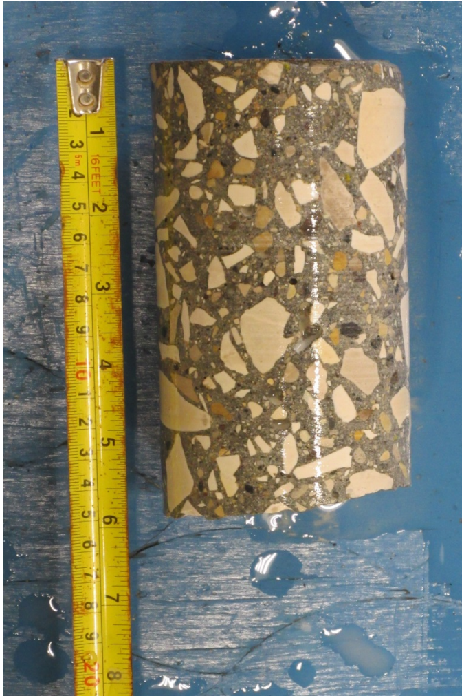
Figure 23 – Core no. A3, east abutment
