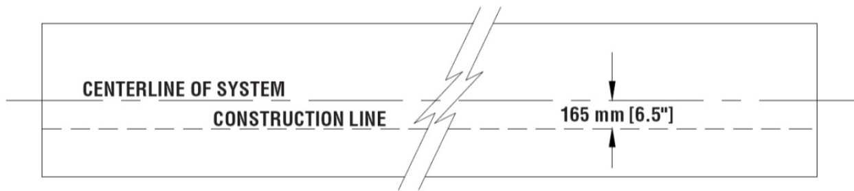
Figure 15 (Top view of concrete foundation)
