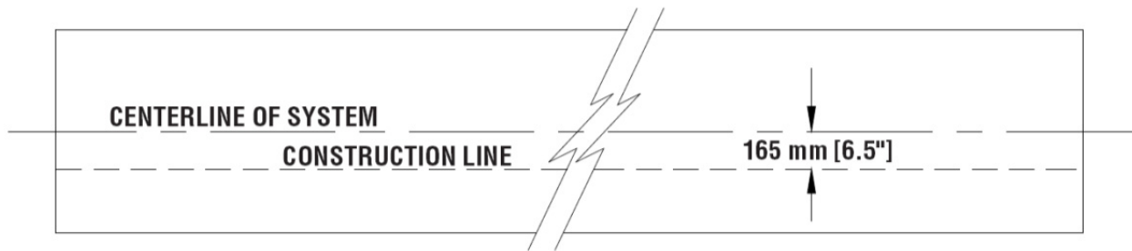
Figure 46 (Top view of concrete foundation)
