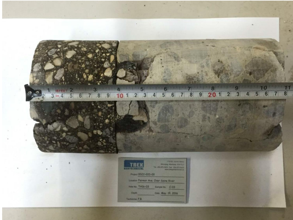
Photo 3: Pavement Core Sample at Test Hole TH16-03
