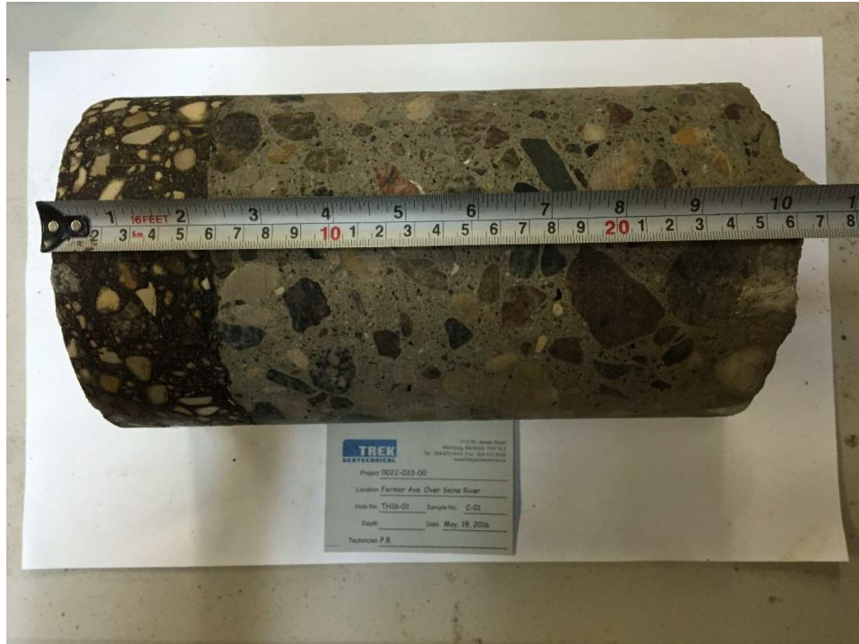
Photo 1: Pavement Core Sample at Test Hole TH16-01
