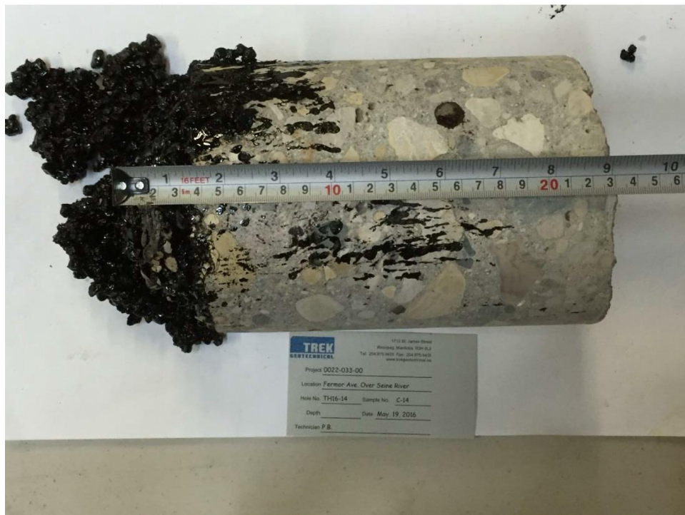
Photo 14: Pavement Core Sample at Test Hole TH16-14
