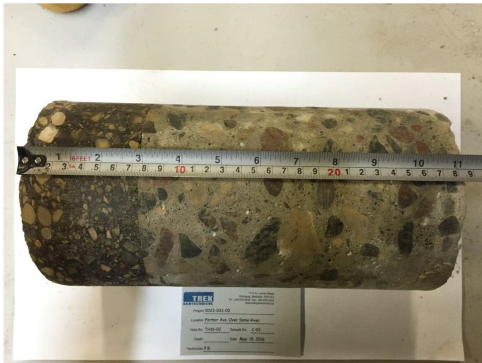
Photo 2: Pavement Core Sample at Test Hole TH16-02
