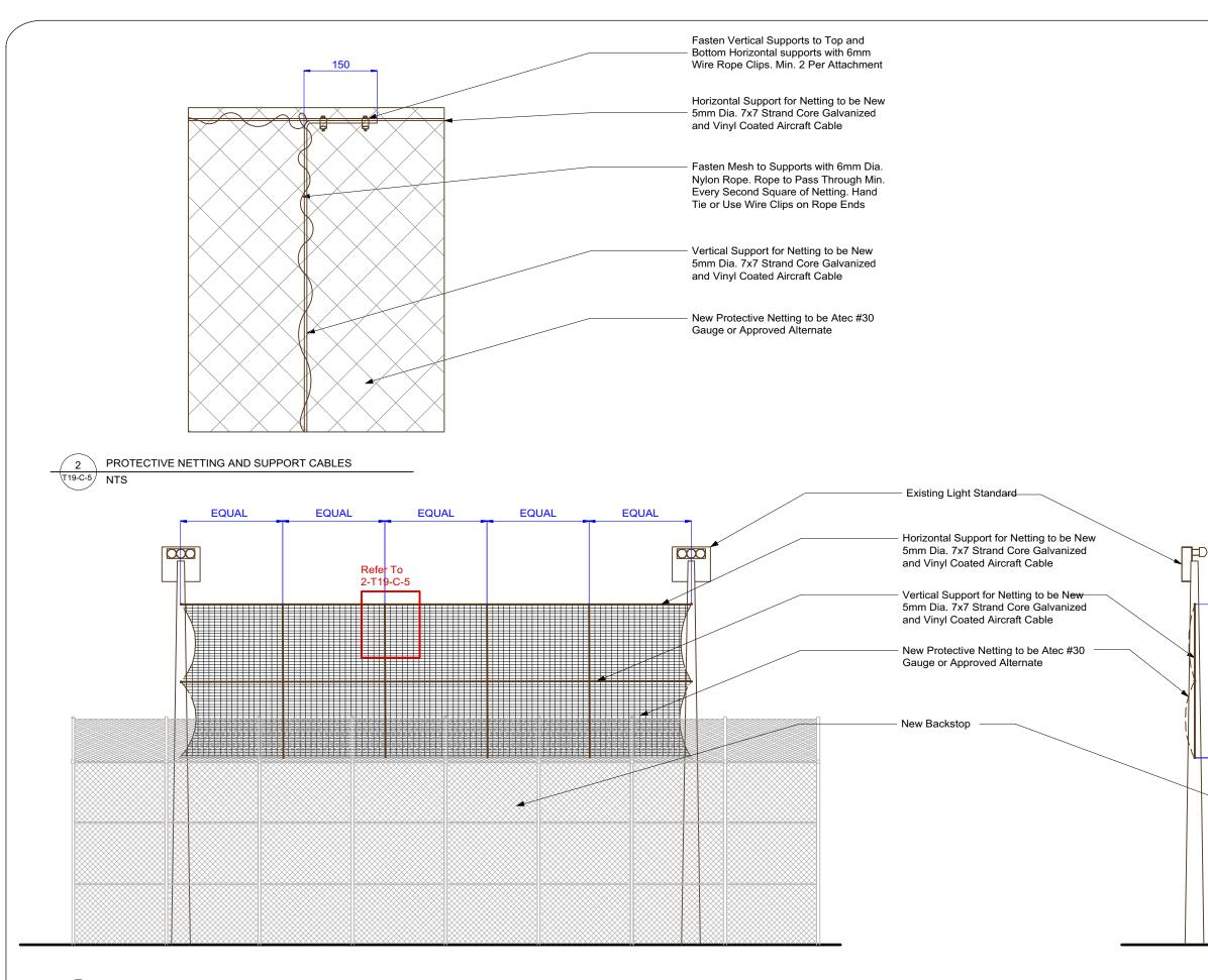
PROTECTIVE NETTING AND SUPPORT CABLES (ELEVATION AND SECTION)
