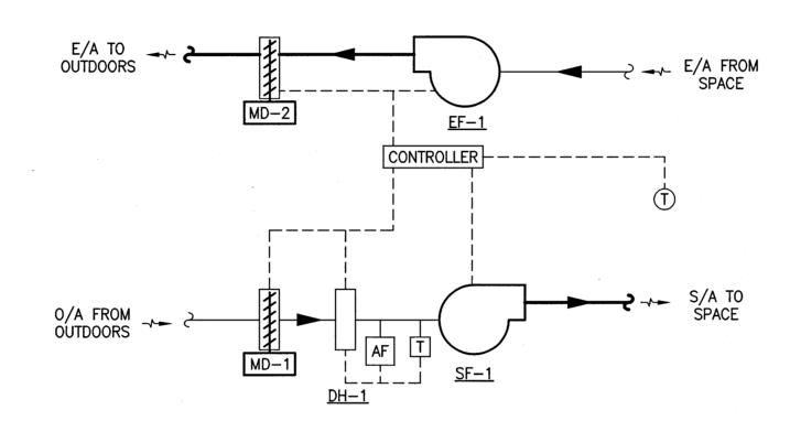
2 RECEIVING/SORTING VENTILATION CONTROL SCHEMATIC SCALE: NTS
