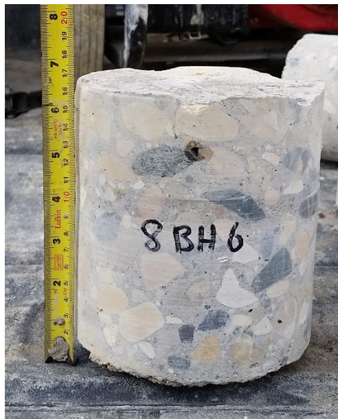
TH01 – 170 mm intact (mislabelled in photo, BH6 = TH01)
