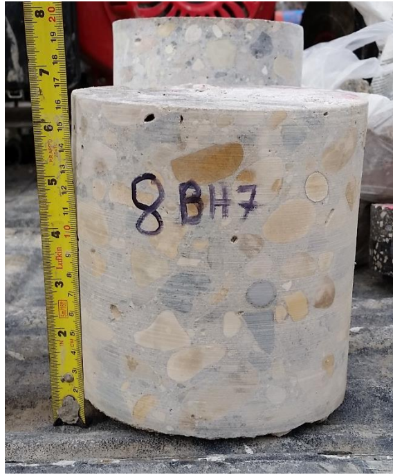
TH02 – 170 mm intact (mislabelled in photo, BH7 = TH02)
