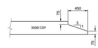
NOTE: ALL NEW CSP'S TO BE INSTALLED C/W BEVELLED END SECTIONS UNLESS NOTED OTHERWISE.
