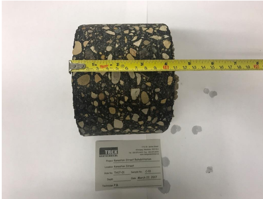
Photo 1: Pavement Core Sample at Test Hole TH17-01
