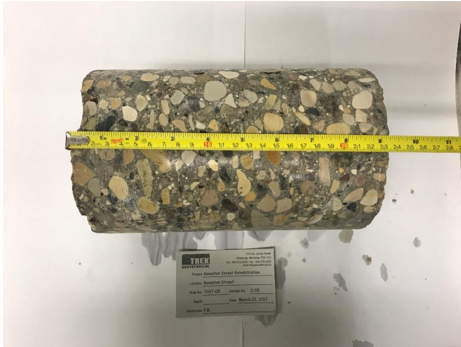
Photo 3: Pavement Core Sample at Test Hole TH17-05
