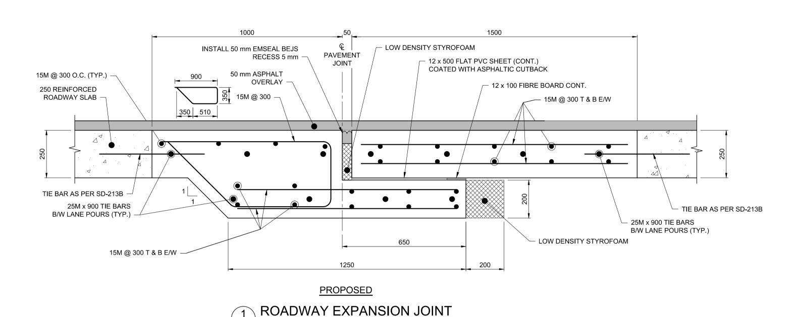
50 WIDE EMSEAL BEJS SAW CUT AND REMOVE CONCRETE - CONCRETE MEDIAN BARRIER FULL DEPTH FOR 50 mm GAP BETWEEN ROADWAY SLABS AND BARRIERS, INSTALL EMSEAL BEJS -RECESS - SPLICE BETWEEN ROADWAY AND BARRIER EMSEAL SECTIONS (TYP.) REINFORCED ROADWAY SLAB SEE "ROADWAY EXPANSION JOINT" SECTION THIS SHEET SEE "ROADWAY EXPANSION JOINT" SECTION THIS SHEET
