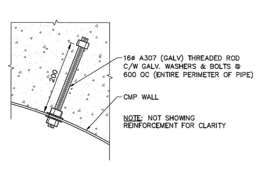
CMP ANCHORING DETAIL SCALE: 1:5
