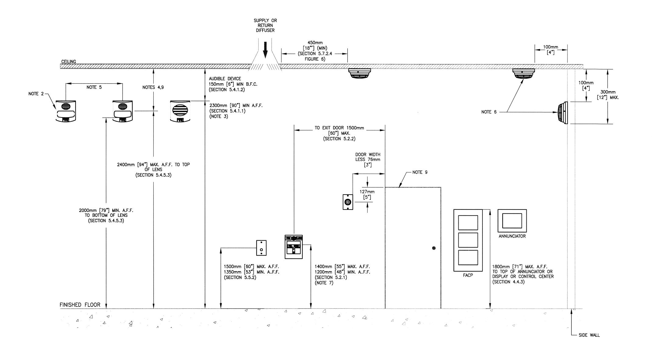
1 FIRE ALARM DEVICE MOUNTING HEIGHT DETAIL (PER CAN/ULC-S524)
