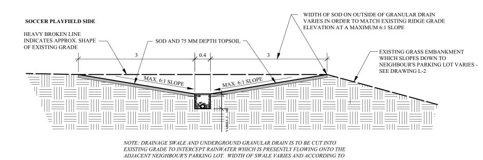
MAX. 6:1 SIDE SLOPES ON THE EMBANKMENT FIELD 2 WEST GRANULAR DRAIN SECTION
