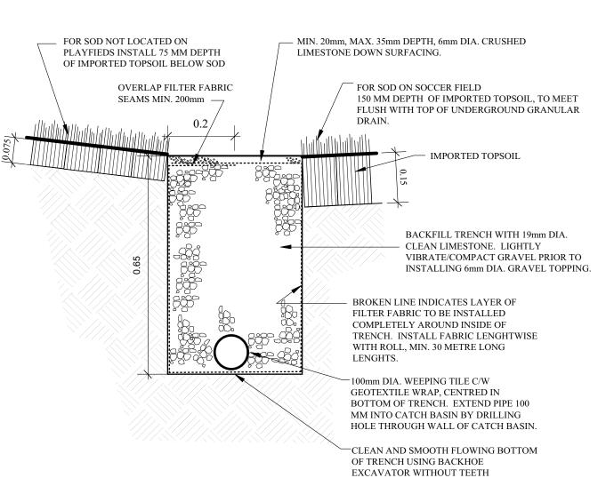
1 UNDERGROUND CHANNEL SECTION @ DEEPER POINT L3 Scale: 1:10
