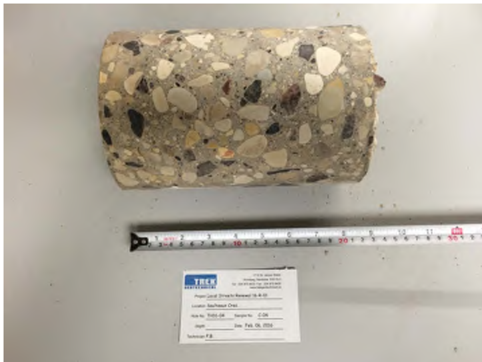
Photo 4: Pavement Core Sample at Test Hole TH16-04
