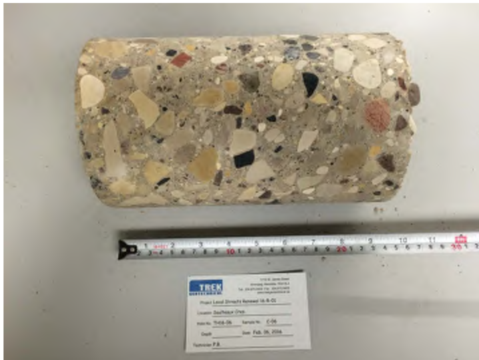
Photo 6: Pavement Core Sample at Test Hole TH16-06
