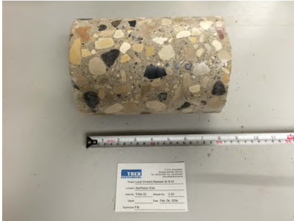
Photo 1: Pavement Core Sample at Test Hole TH16-01
