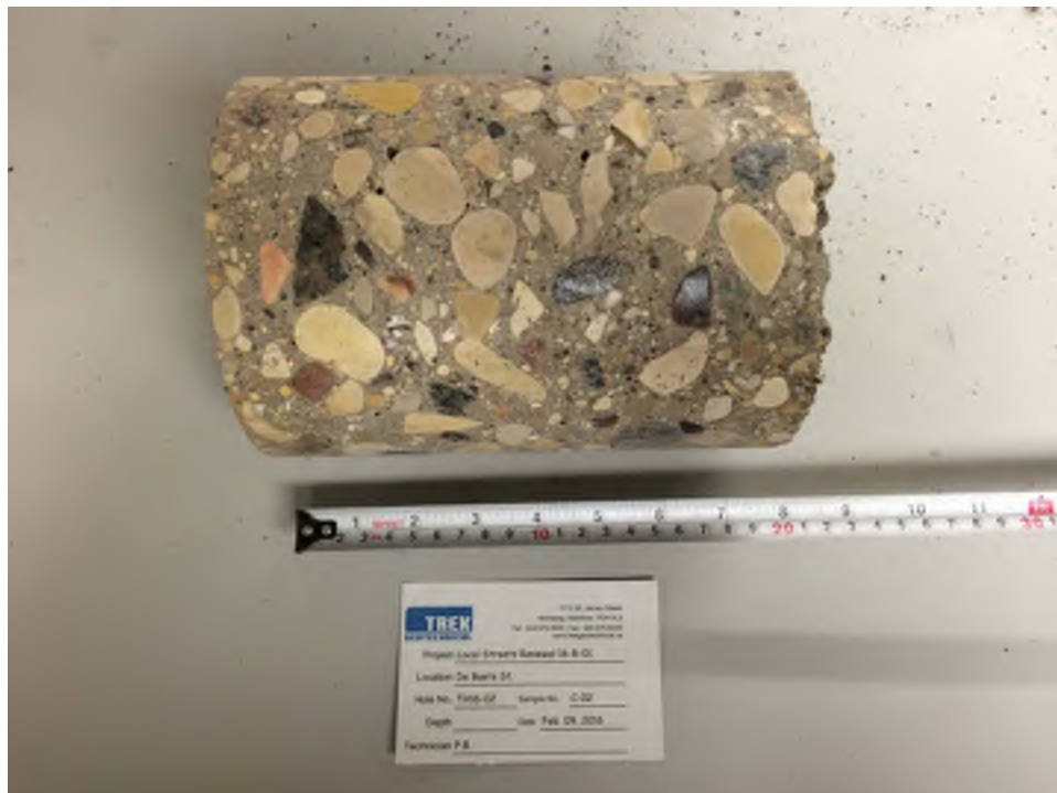
Photo 2: Pavement Core Sample at Test Hole TH16-02
