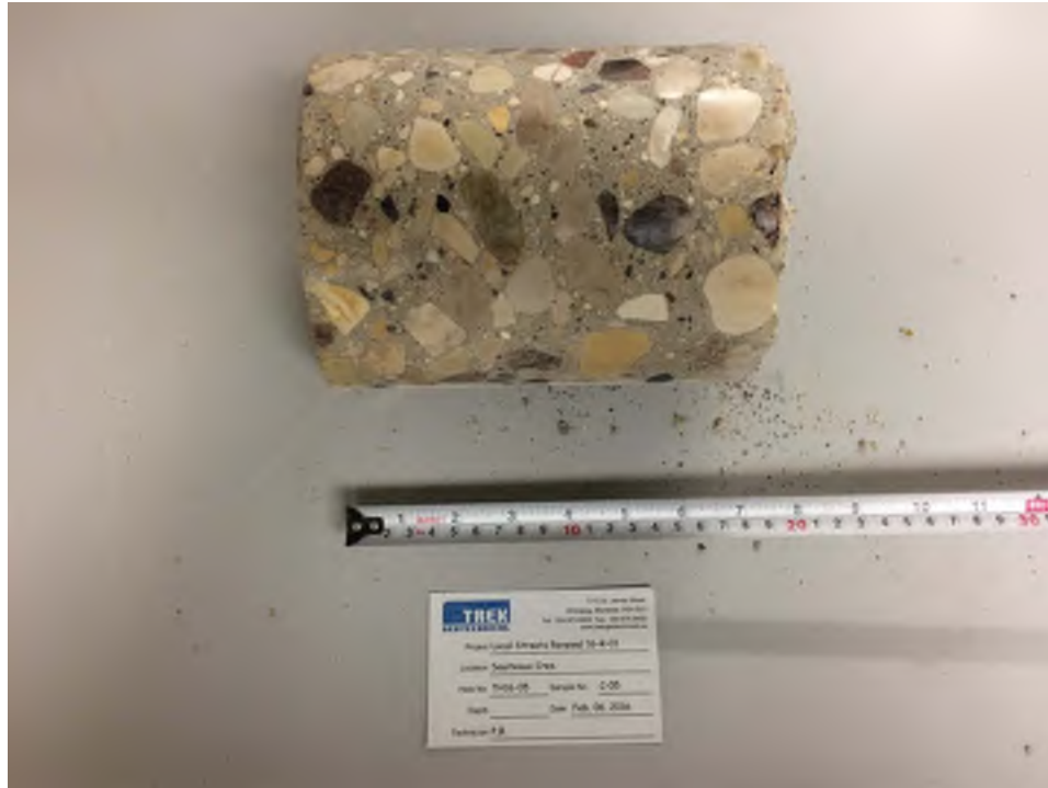
Photo 5: Pavement Core Sample at Test Hole TH16-05
