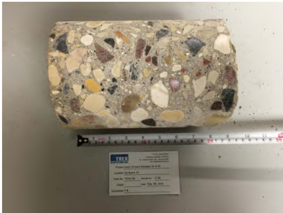
Photo 6: Pavement Core Sample at Test Hole TH16-06
