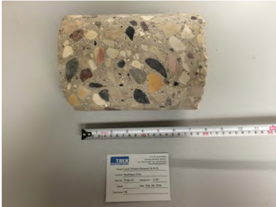
Photo 7: Pavement Core Sample at Test Hole TH16-07
