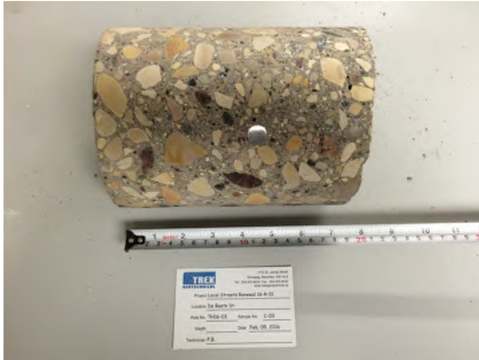
Photo 3: Pavement Core Sample at Test Hole TH16-03
