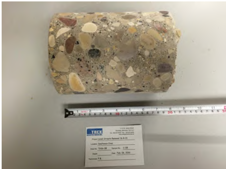
Photo 8: Pavement Core Sample at Test Hole TH16-08
