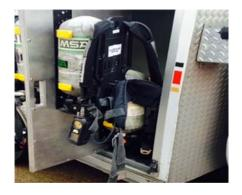
a) The Equipment Area Cabinets shall be designed to accommodate a back board and stretcher, fire fighter turnout gear, fire extinguisher, various loose fire equipment and must have a sliding SCBA bracket.
