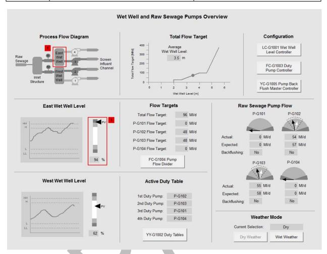
Figure 2-3: Sample Process Equipment Overview Display
