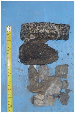
Core sample from Testhole TH5
