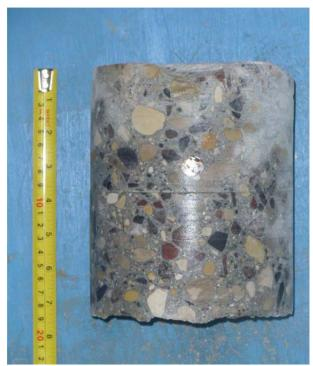
Core sample from Testhole TH1
