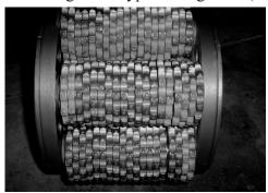
Figure 9 – Grinder Cutting Head
