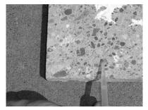
Place a drop of clean drinking or distilled water on the pavement surface.
