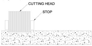
**Figure 2 - Initial Pass, Intersection Groove Cut** After the first pass, one stop will sit on the old pavement surface and the other stop will sit in the newly cut groove (Figure 3). This produces ridges which are unacceptable.
