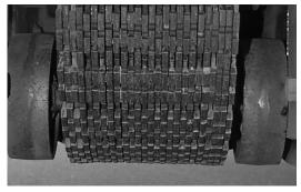
Figure 4 – Saw Blade Cutting Head
