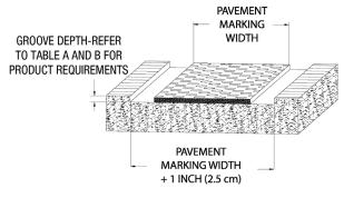
Figure 1 – Groove and Pavement Marking – Typical Section
