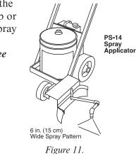
*Note:* If you are using tape wider than 4 inches, **spray multiple passes, overlapping the previous pattern by 1-2"**. Allow additional time for overlapped areas to set. See Appendix B to determine the amount of adhesive that is needed to cover a specific area.
