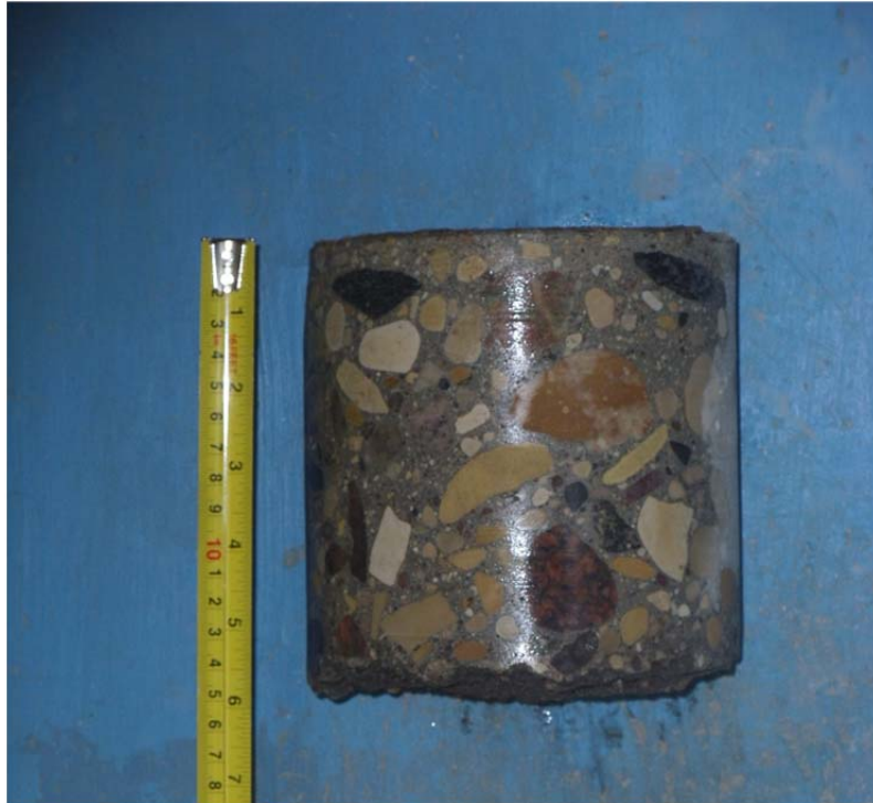
Core sample from Testhole TH1
