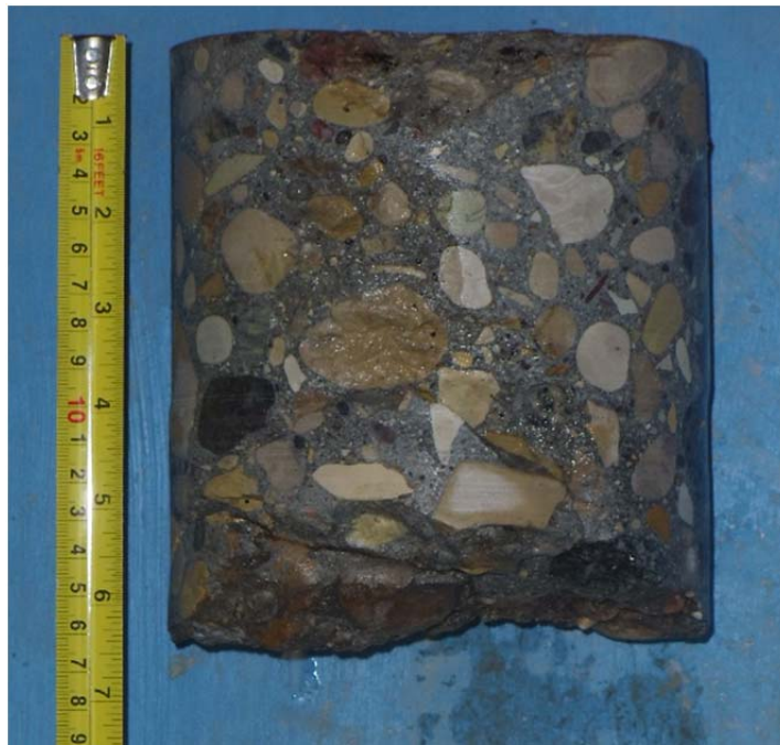
Core sample from Testhole TH6
