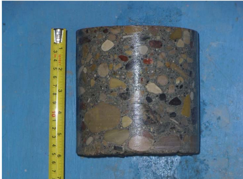
Core sample from Testhole TH1
