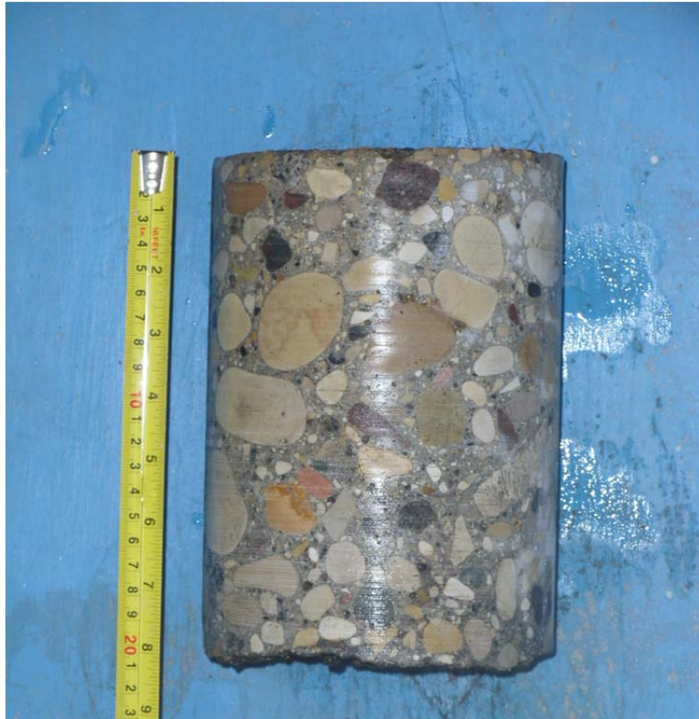
Core sample from Testhole TH3
