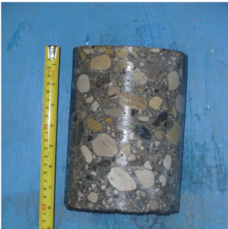
Core sample from Testhole TH1
