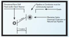
When the minimum 1 metre horizontal separation is not maintained, conductor or pipeline must be continuously exposed.
