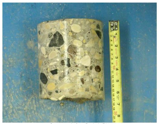
Core sample from Testhole TH4
