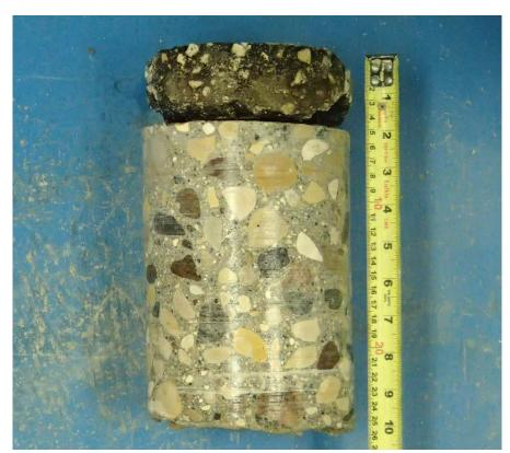
Core sample from Testhole TH3
