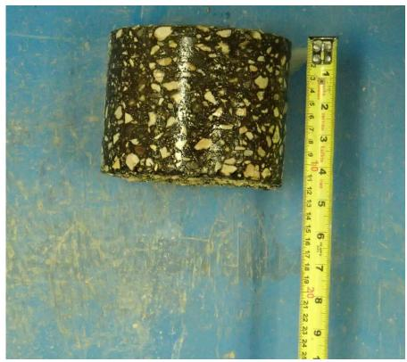
Core sample from Testhole TH3
