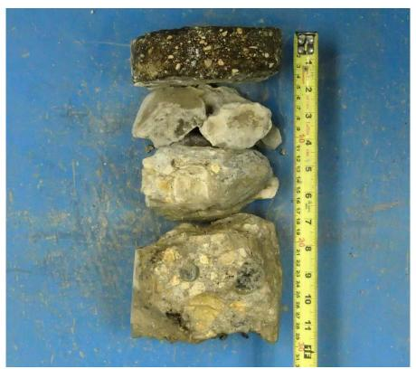
Core sample from Testhole TH1
