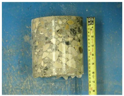
Core sample from Testhole TH4
