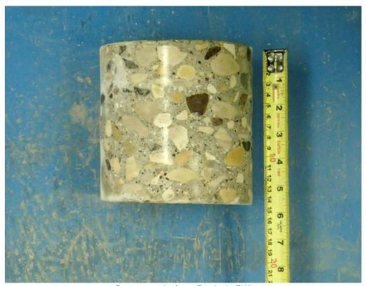
Core sample from Testhole TH2
