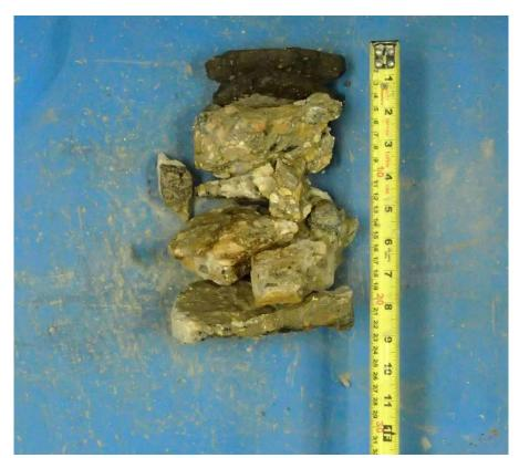
Core sample from Testhole TH5
