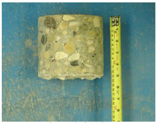
Core sample from Testhole TH2
