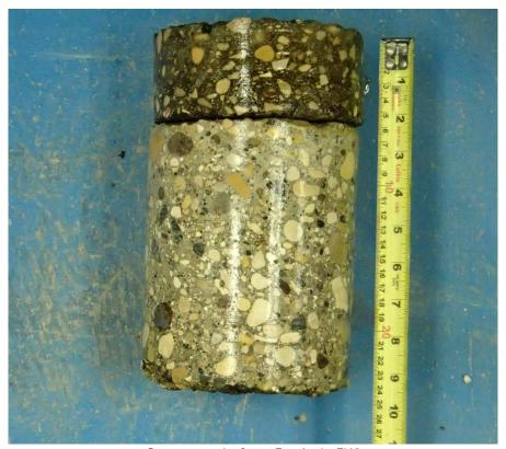
Core sample from Testhole TH2
