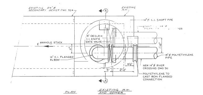
INV. EL 740.39 FOLTETHYLENE TO CAST IRON FLANGED CONNECTION ---48" MANHOLE - 14" Ø POLYETHYLENE PIPE BRACKET -INV. E.L. 730.43 EXISTING 14"
