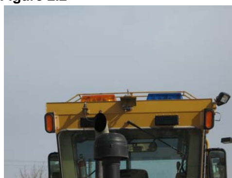
Figure 2.1 and 2.2: Motor Grader with roof mounted dual rotating halogen beacons, slow moving vehicle sign, and caution signage.
