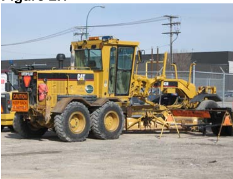
Figure 2.1 and 2.2: Motor Grader with roof mounted dual rotating halogen beacons, slow moving vehicle sign, and caution signage.
