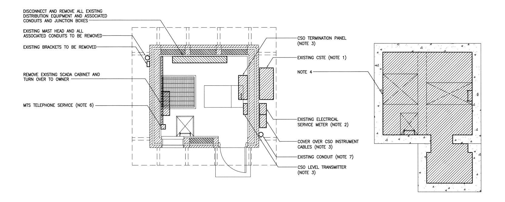
ELECTRICAL ROOM FLOOR PLAN SCALE: 1:40
