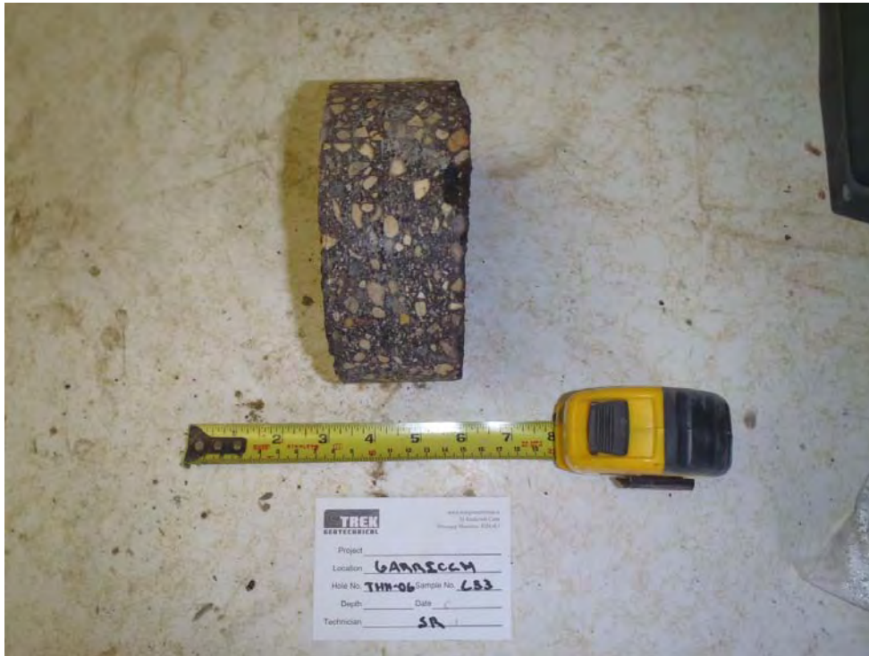
Photo 11: Asphalt core sample from TH11-06
