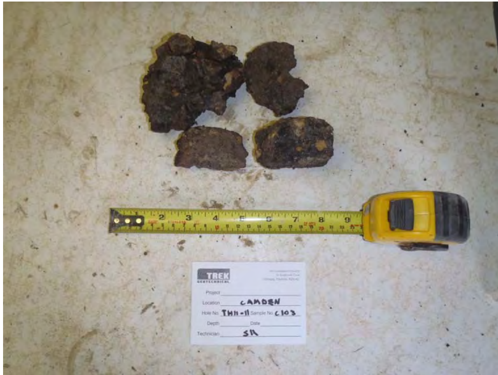
Photo 21: Asphalt core sample from TH11-11
