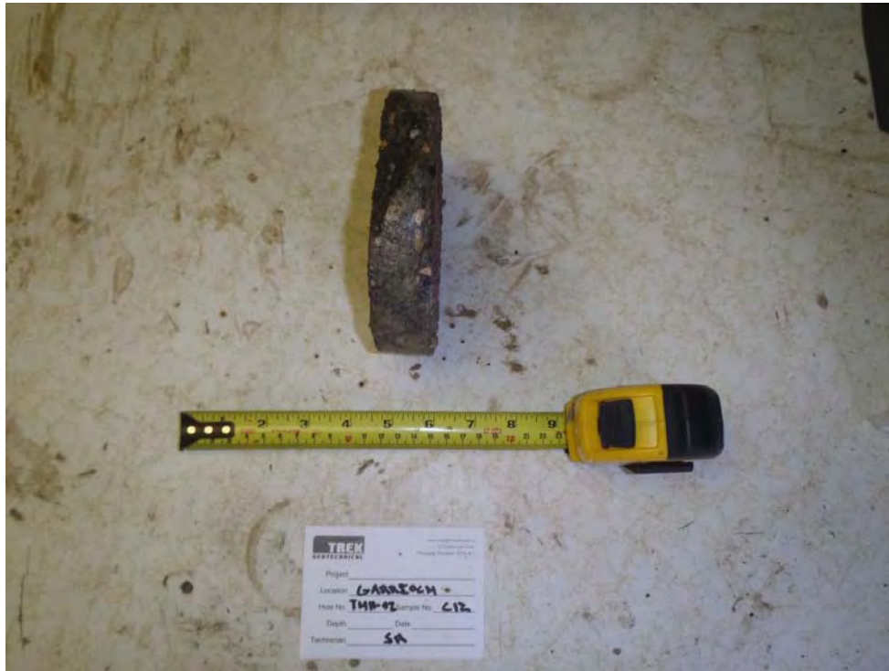
Photo 3: Asphalt core sample from TH11-02
