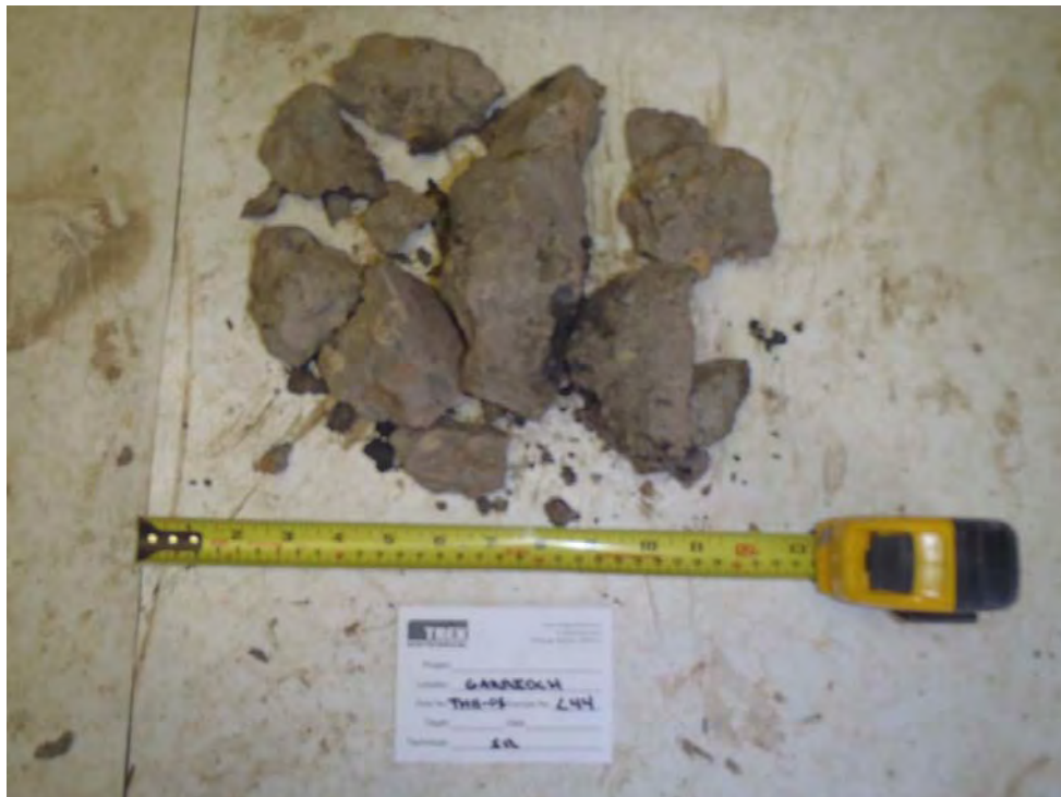
Photo 10: Concrete core sample from TH11-05
