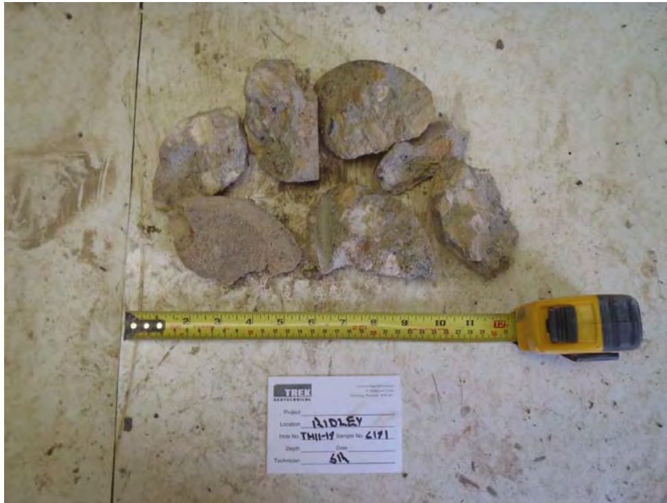
Photo 29: Concrete core sample from TH11-19
