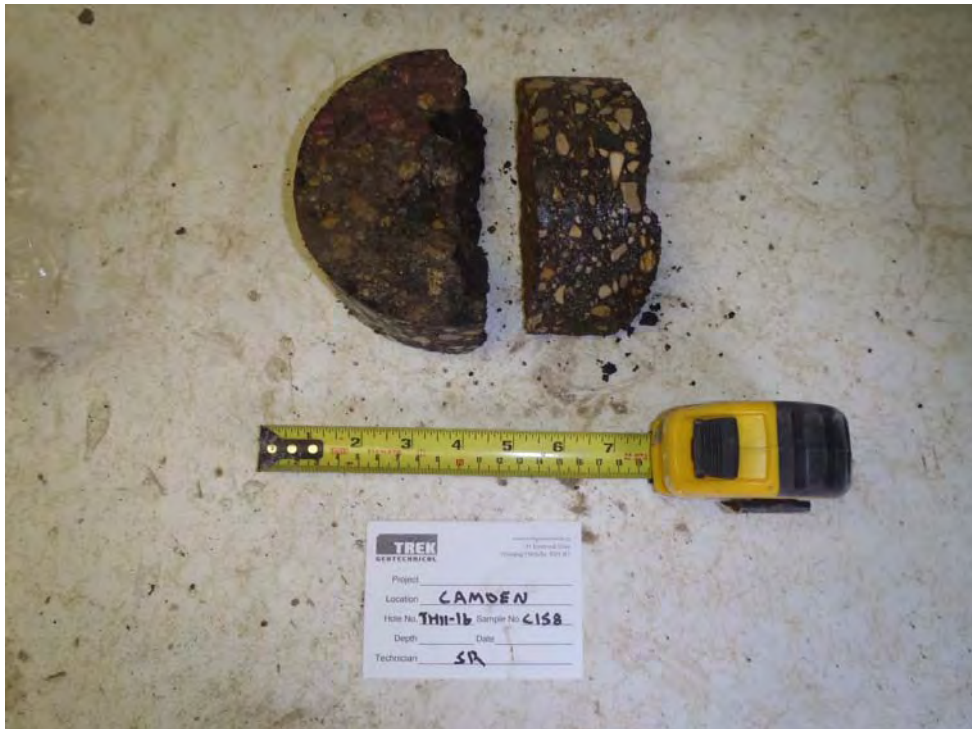
Photo 26: Asphalt core sample from TH11-16
