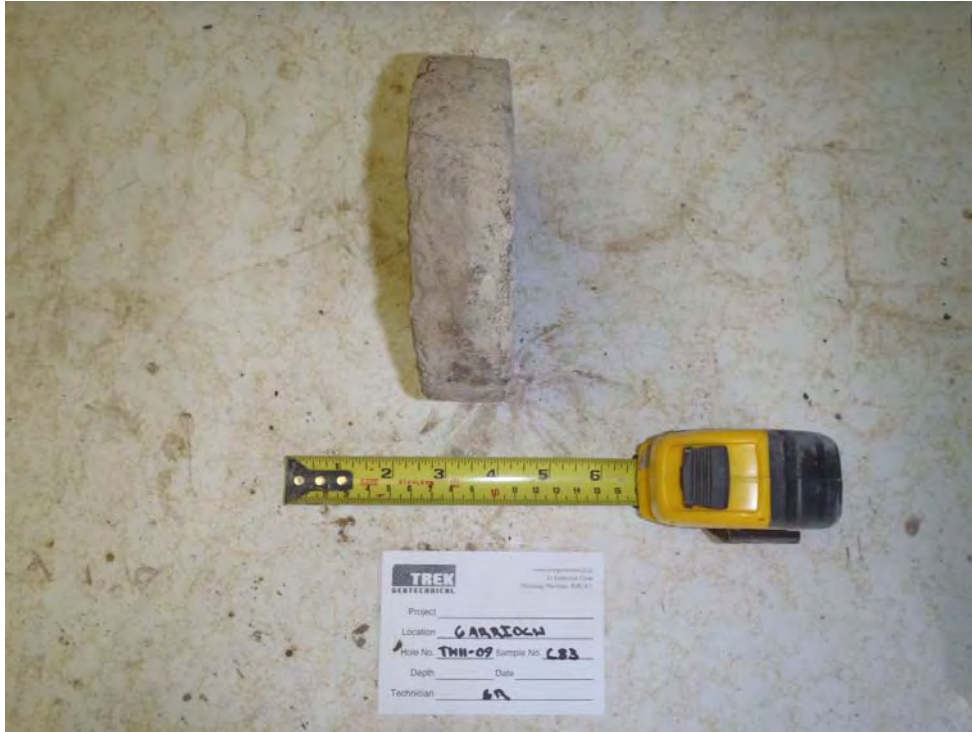
Photo 17: Asphalt core sample from TH11-09
