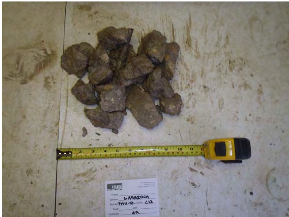
Photo 4: Concrete core sample from TH11-02
