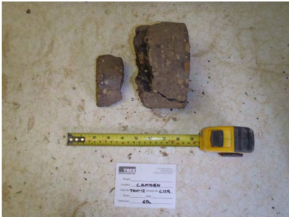
Photo 22: Asphalt core sample from TH11-12
