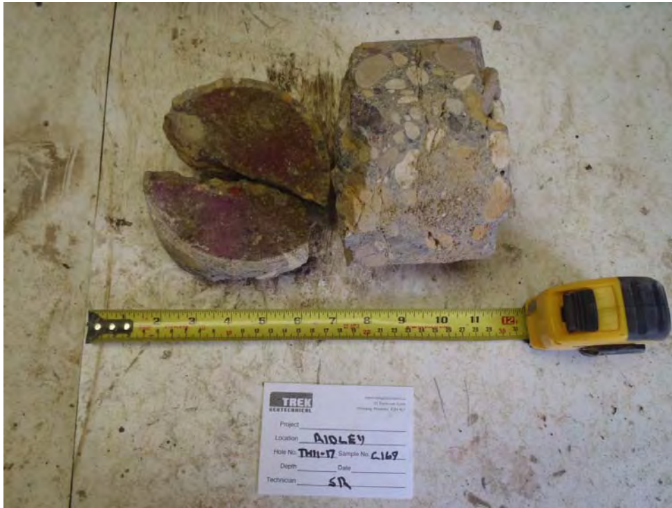
Photo 27: Concrete core sample from TH11-17
