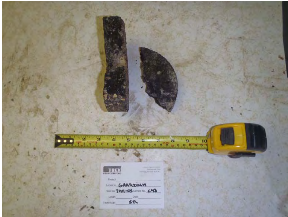
Photo 9: Asphalt core sample from TH11-05
