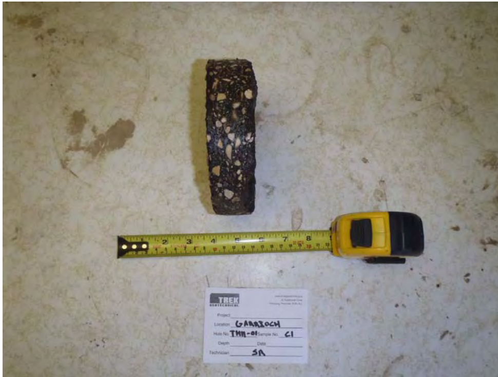
Photo 1: Asphalt core sample from TH11-01
