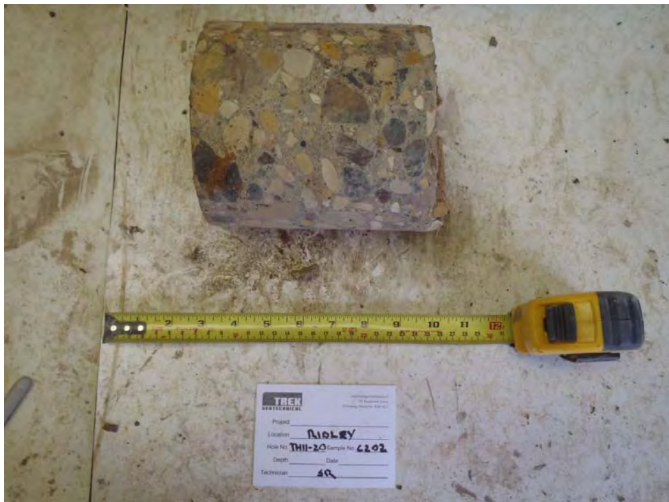
Photo 30: Concrete core sample from TH11-20
