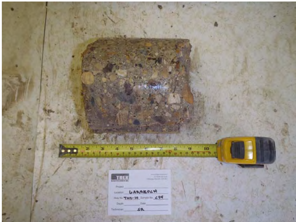
Photo 20: Concrete core sample from TH11-10
