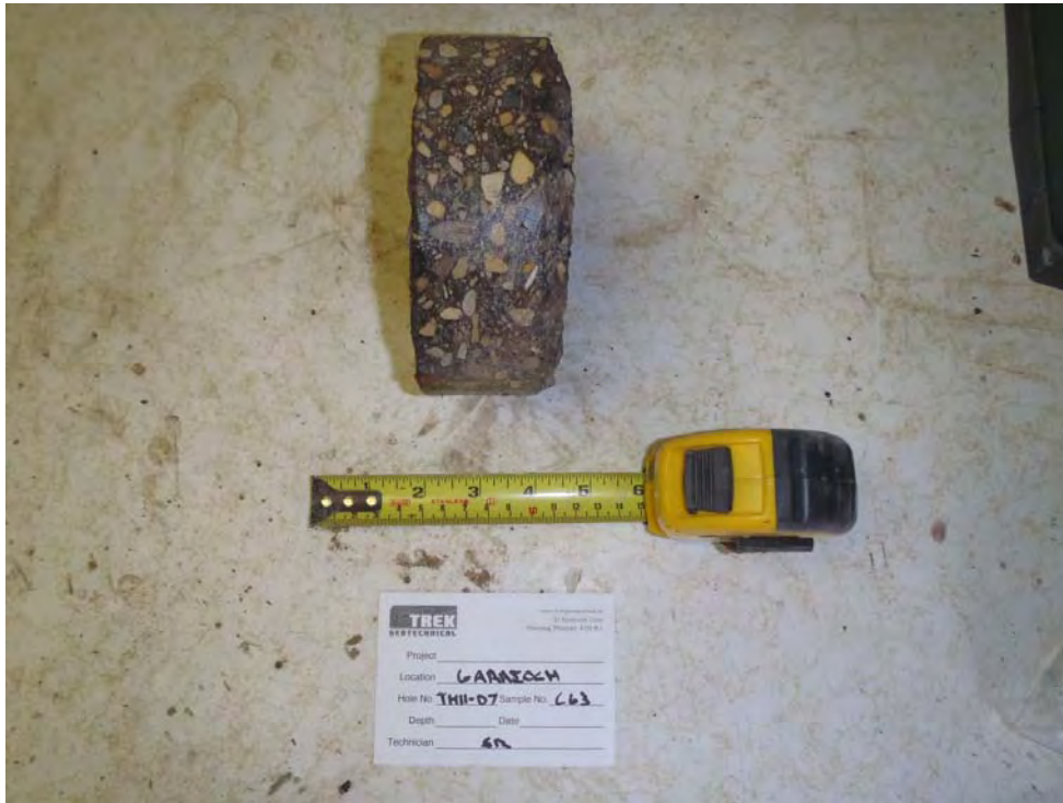
Photo 13: Asphalt core sample from TH11-07
