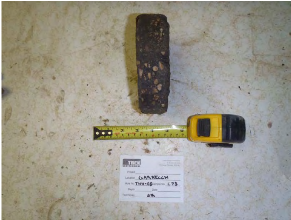
Photo 15: Asphalt core sample from TH11-08
