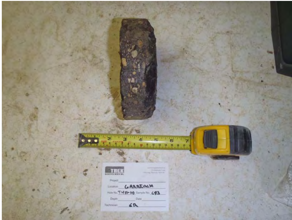
Photo 19: Asphalt core sample from TH11-10
