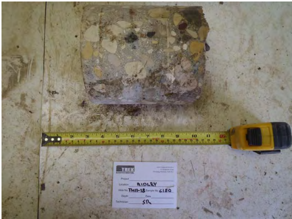
Photo 28: Concrete core sample from TH11-18
