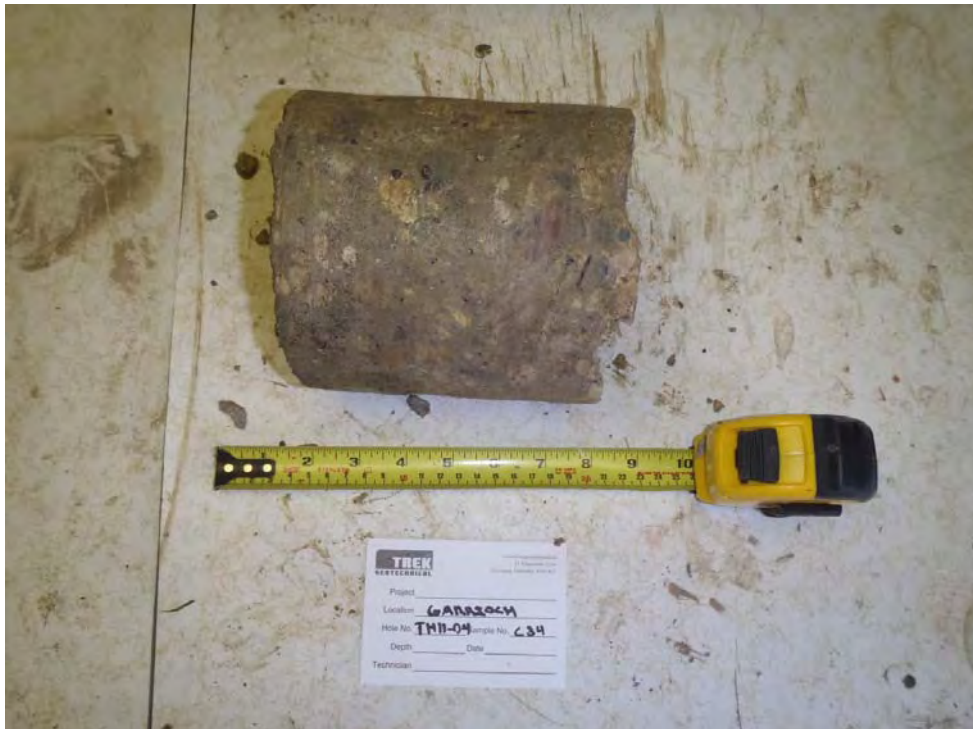
Photo 8: Concrete core sample from TH11-04
