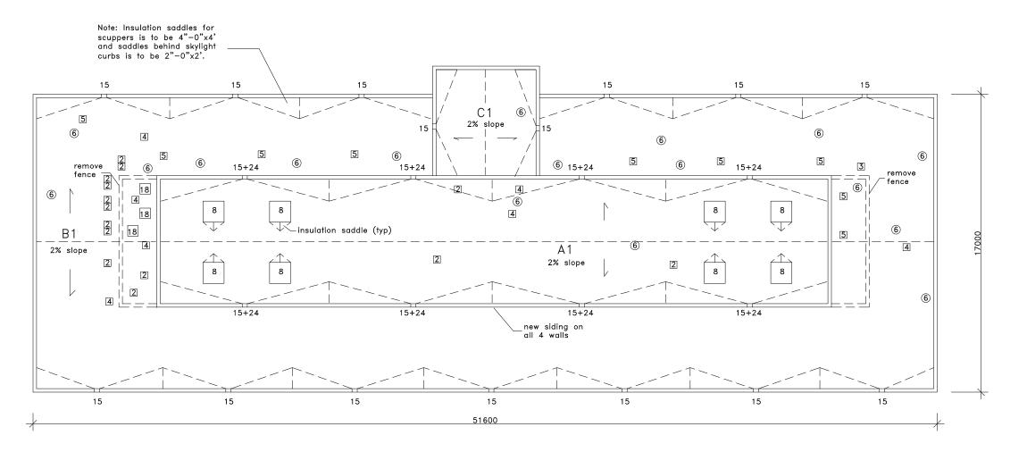
Note: Allow for the new siding band on the walls of area A1 is to extend to 8" above the top of the new roofing on areas C1 and B1. The siding on area B1 is to extend to the bottom of the overhang. On area C1 the siding is to also extend to the bottom of the overhang but to the top of the beams on the side walls. Final layout is to be confirmed on site with the Contract Administrator.
