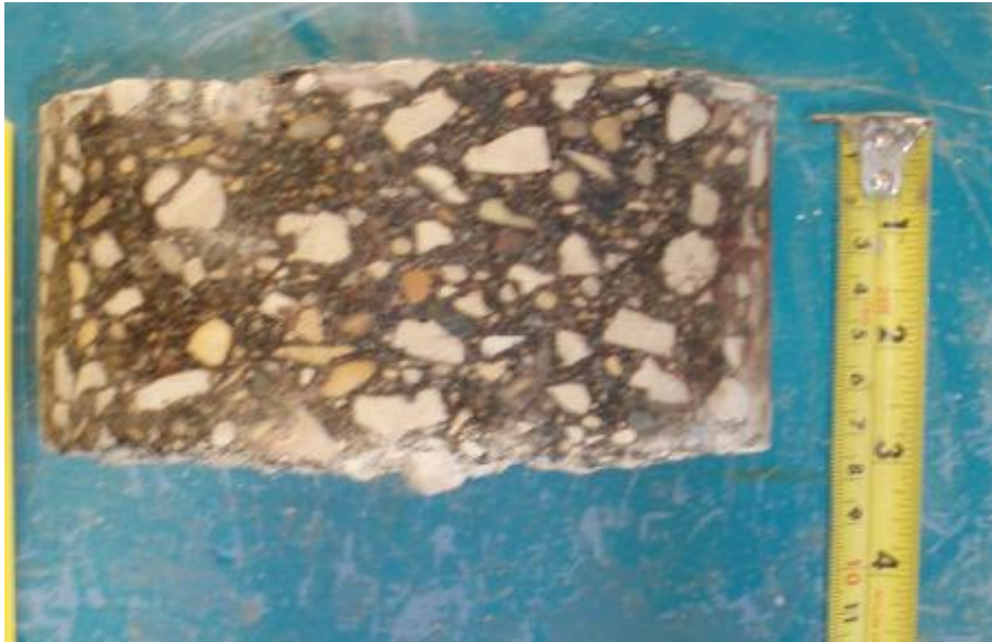
Core sample for Testhole TH1
