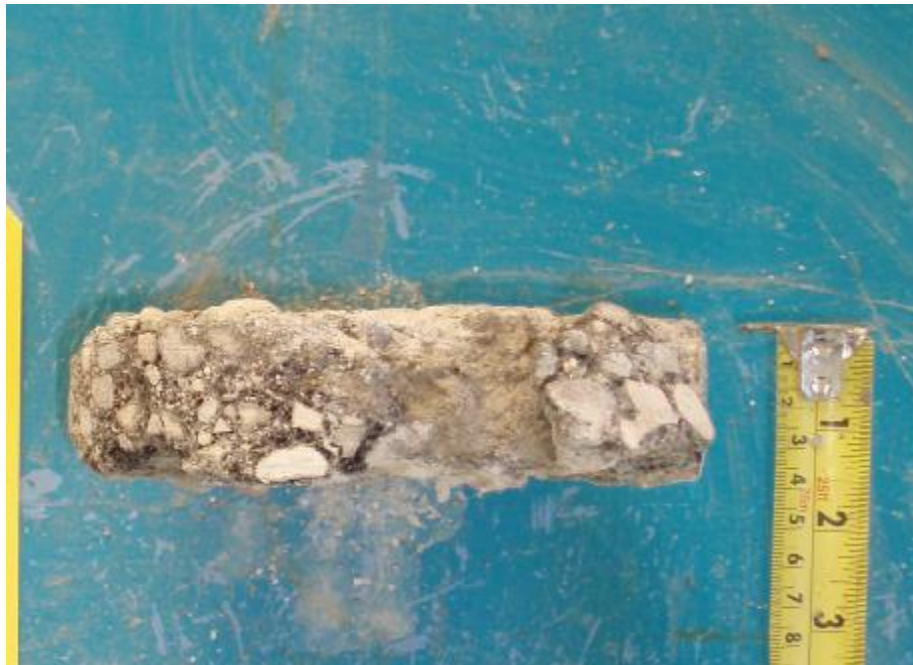
Core sample for Testhole TH2
