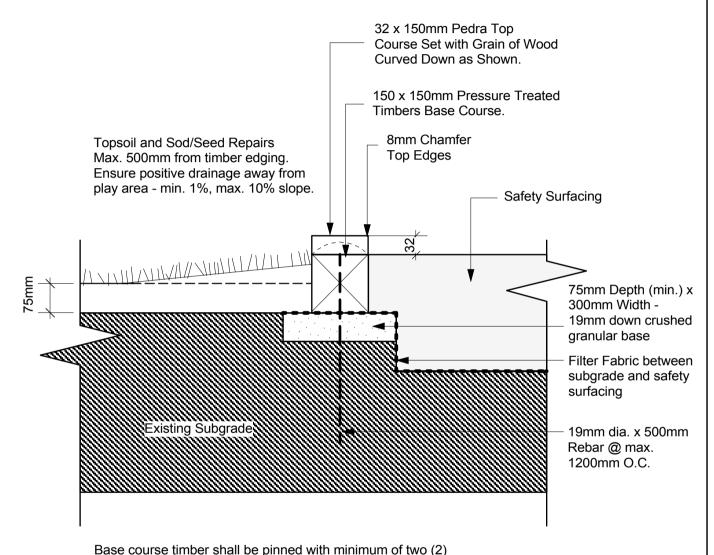
19mm dia. rebar @ max. 1200mm O.C.
