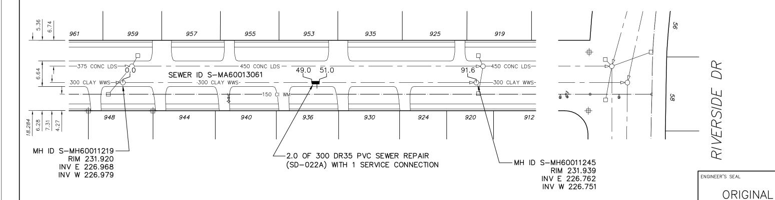
SEWER JUNCTION INFORMATION FROM SEWER VIDEO INSPECTION SEWER ID S-MA60013061 DISTANCE FROM MH ID S-MH60011219 50.4 E 100ø SOUTH CNI
