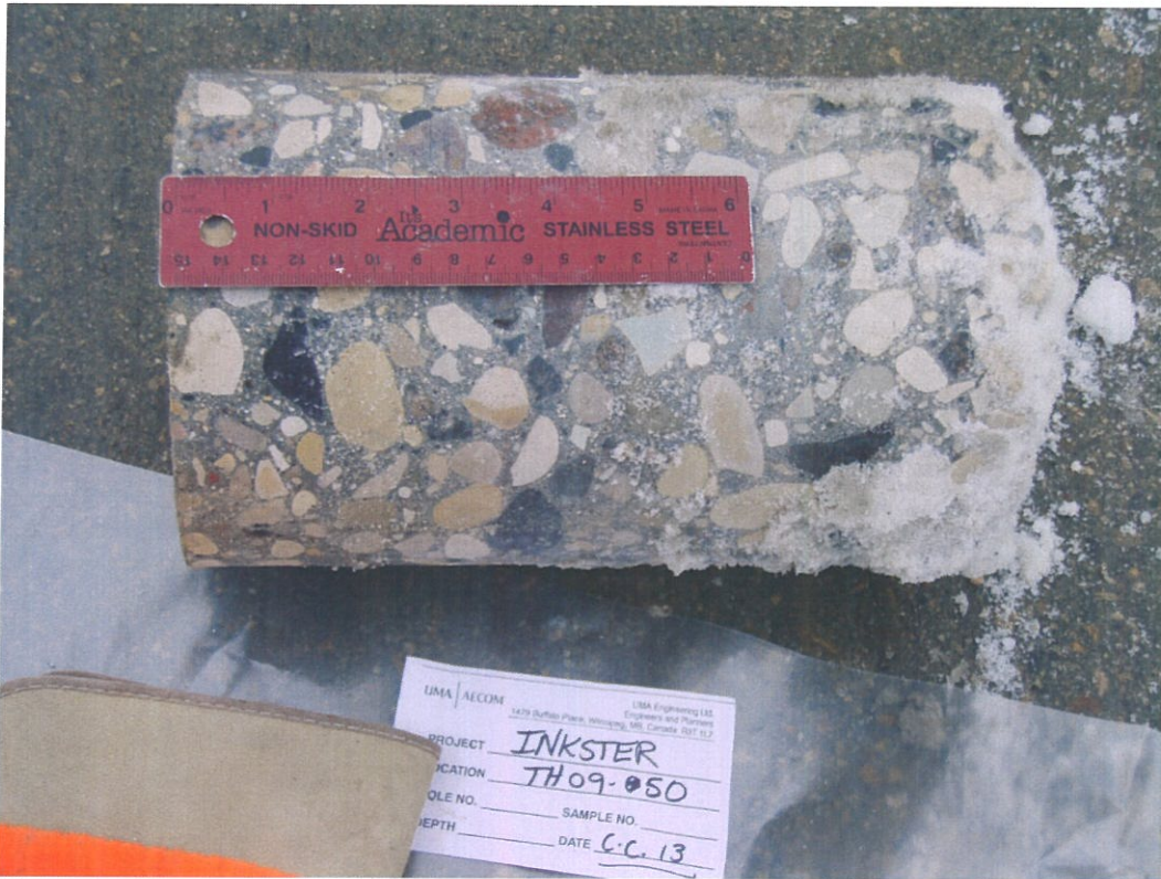
Photo 33: Core sample from TH-09-50
