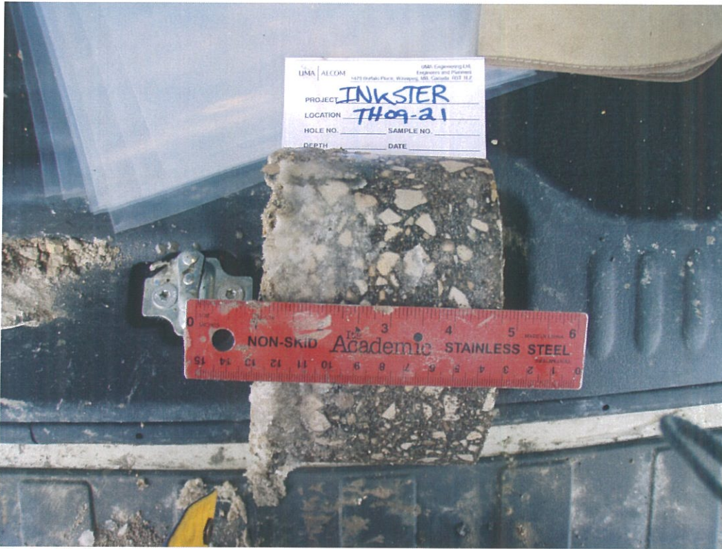
Photo 15: Core sample from TH-09-21
