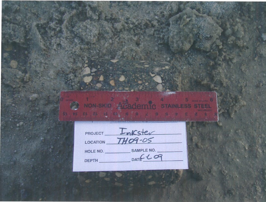
Photo 5: Core sample from TH-09-05
