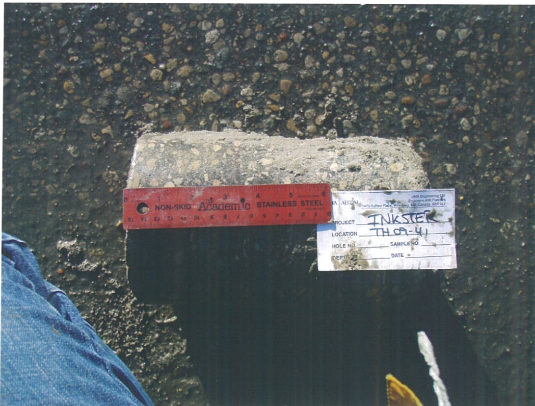
Photo 28: Core sample from TH-09-41
