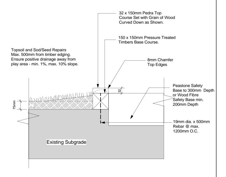
Base course timber shall be pinned with minimum of two (2) 19mm dia. rebar @ max. 1200mm O.C. Pedra top course shall be screwed down using stainless steel or ceramic-coated screws and sized to suit. Two screws at each end and every 600mm alternating sides along length. Min. length of timbers to be 1200mm. Install longest lengths possible.
