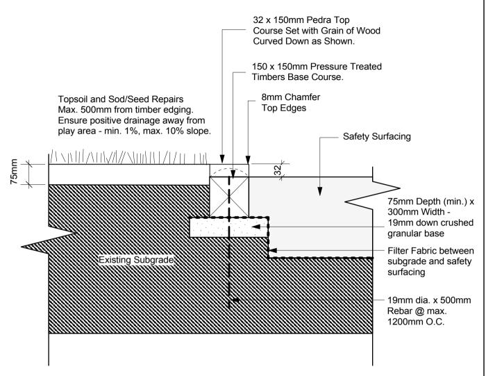
Base course timber shall be pinned with minimum of two (2) 19mm dia. rebar @ max. 1200mm O.C.
