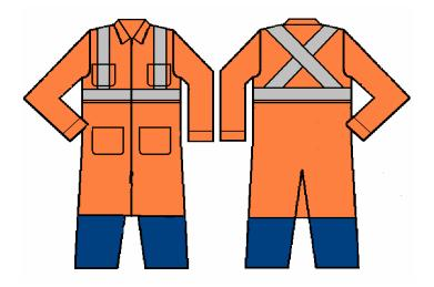
E9.5 In reference to E2.9 (Item No. 8), the reflective positioning requirements are shown below:
