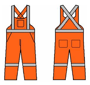
E9.4 In reference to E2.6 (Item No. 5), the reflective positioning requirements are as shown below:
