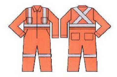
E9.3 In reference to E2.5 (Item No. 4), the reflective positioning requirements are as shown below:
