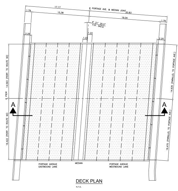
AREAS TO APPLY METHACRYLATE CRACK SEALER
