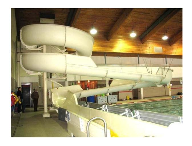
EKW- PHOTO 9: EXISTING WATERSLIDE SEEN LOOKING SOUTH. THE WATERSLIDE INCLUDING THE MAST AND SUPPORT STRUCTURES ARE TO BE DEMOLISHED AND REMOVED UNDER THIS CONTRACT.
