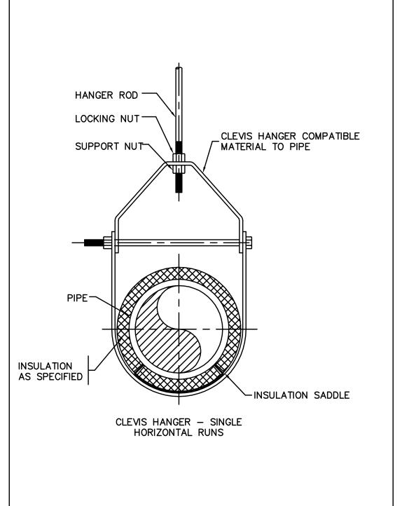
PIPE CLEVIS HANGER DETAIL 2 LOWER ATTACHEMENT
