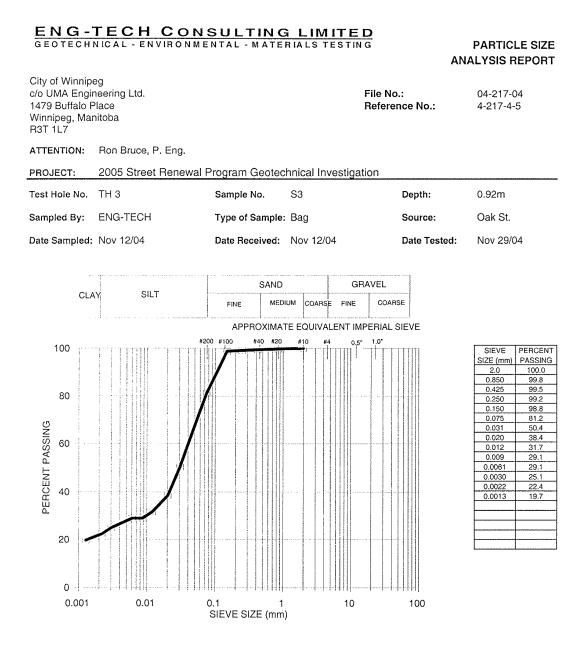
Percent of: GRAVEL (0.0%), SAND (18.8%), SILT (59.3%) and CLAY (21.9%) Sample Description: Clayey Silt, medium plastic, soft, moist, light brown, with clay, some sand sizes.
