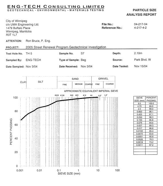
Percent of: GRAVEL (0.1%), SAND (5.3%), SILT (20.7%) and CLAY (73.9%) Sample Description: Clay, high plastic, stiff to firm, moist, dark brown, with silt, trace sand and gravel sizes.
