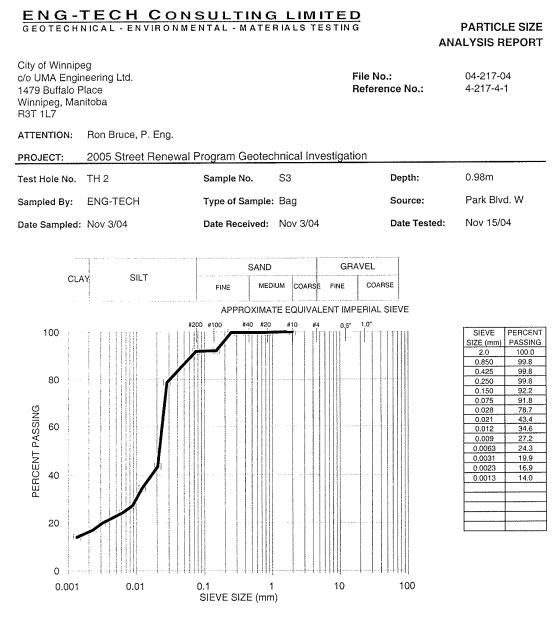
GRAVEL (0.0%), SAND (8.2%), SILT (75.6%) and CLAY (16.2%) tion: Silt, low plastic, soft, moist, light brown, some clay, Percent of: Sample Description: trace sand sizes.
