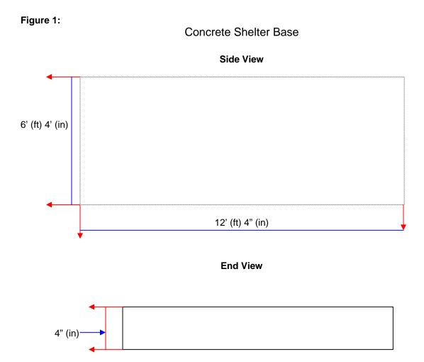
Note: the rebar shall be 5/8" (in) and set at the half way measurement 2" (in) mark in one (1) foot grids.
