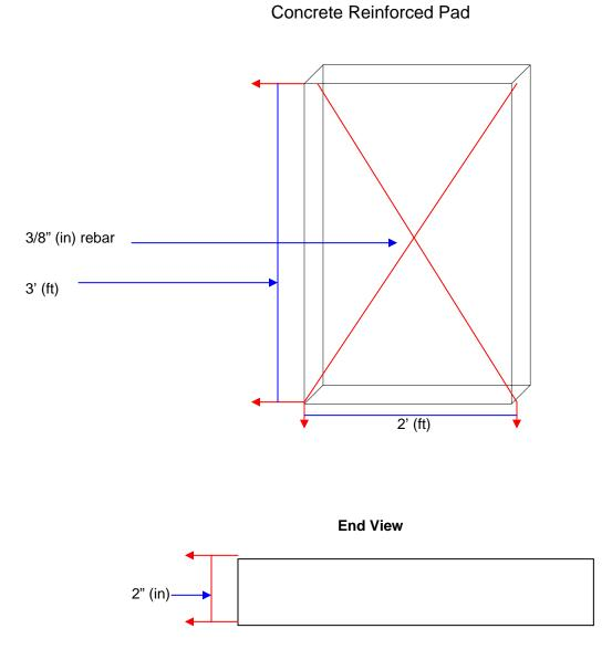
Note: 3/8" (in) rebar to be used as illustrated; to reinforce the concrete non-slip surface is required.
