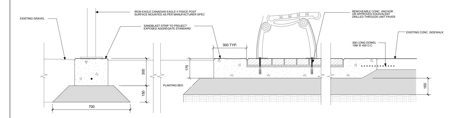
SECTION THROUGH PAVING AREA
